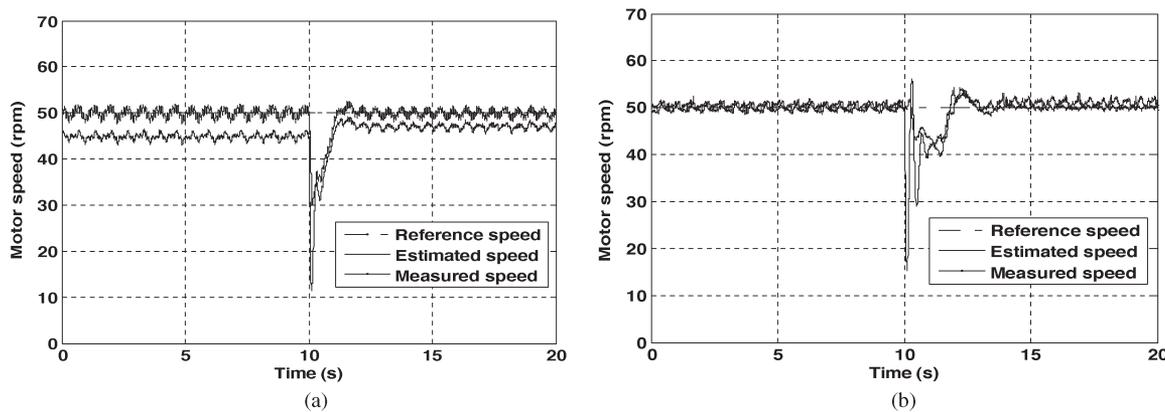
Fig. 11. Sensorless performance for benchmark test 4, at 20% load torque rejection, at 50 r/min. Speed: (a) conventional MRAS. (b) NN MRAS.
