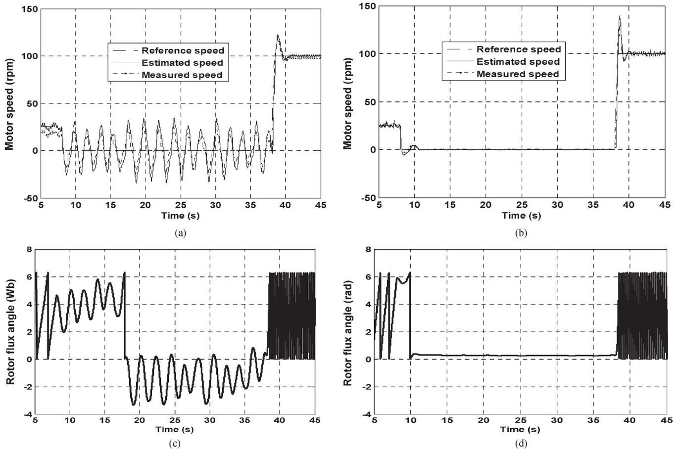
Fig. 9. Sensorless result of benchmark test 2, at no load. Speed: (a) conventional MRAS. (b) NN MRAS. Rotor flux position: (c) conventional MRAS. (d) NN MRAS.
