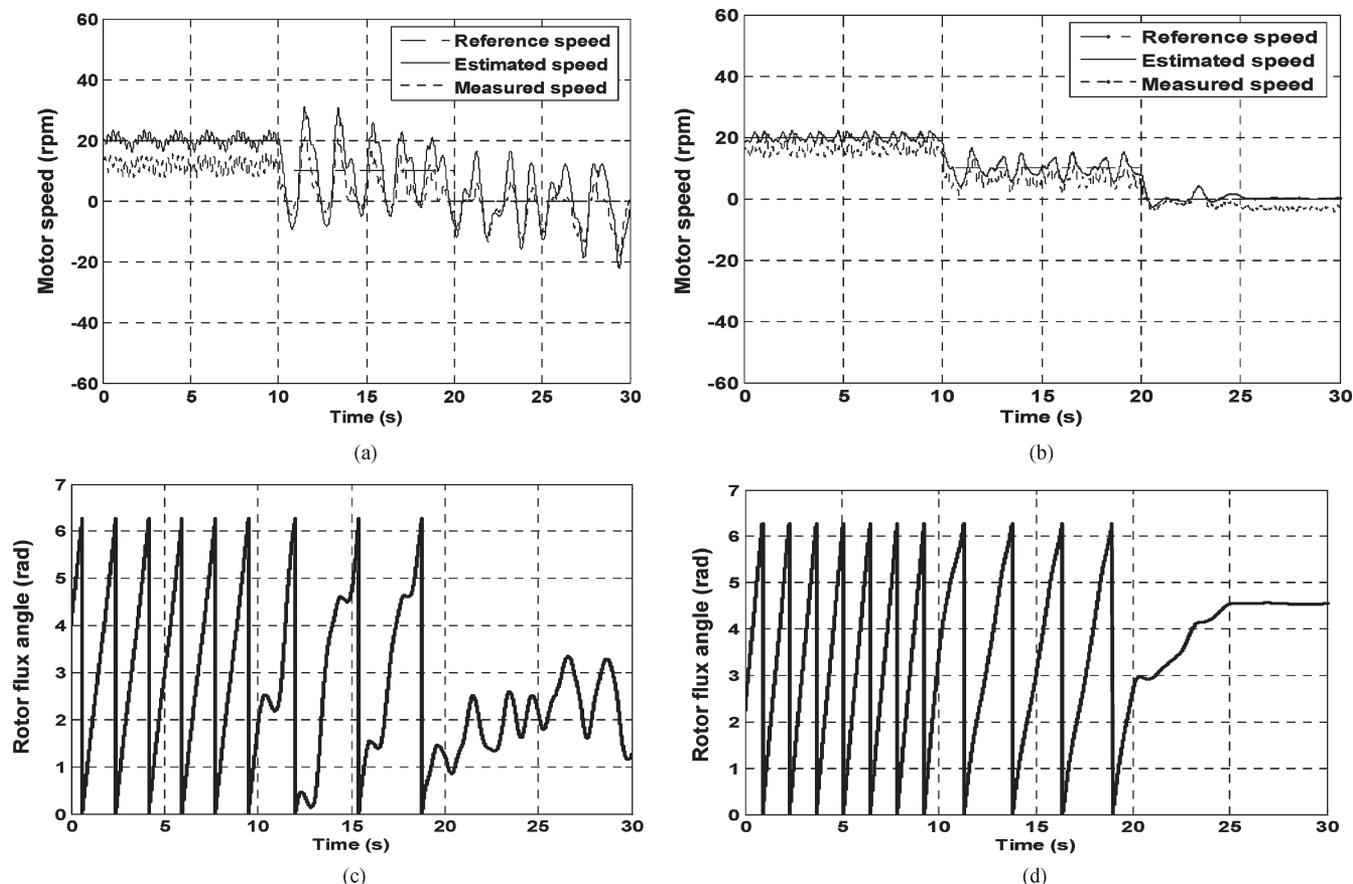
Fig. 10. Sensorless result of benchmark test 3, at 10% load. Speed: (a) conventional MRAS. (b) NN MRAS. Rotor flux position: (a) conventional MRAS. (b) NN MRAS.
