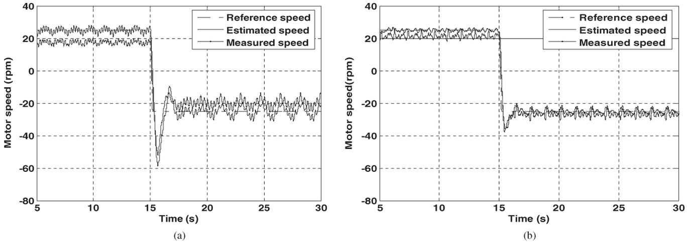
Fig. 12. Sensorless performance for benchmark test 5, at  $\pm 25$  rpm speed reversal, at 10% load. Speed: (a) conventional MRAS. (b) NN MRAS.
