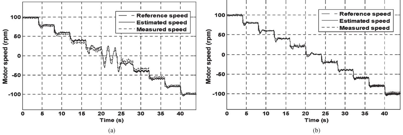
Fig. 8. Sensorless performance for benchmark test 1, at no load. Speed: (a) conventional MRAS. (b) NN MRAS.
