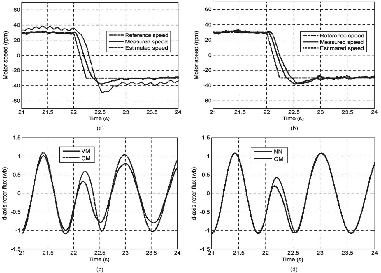
Fig. 5. Open-loop speed reversal from 30 to  $-30$  r/min, at 10% load. Speed: (a) conventional MRAS. (b) NN MRAS. Model outputs: (c) conventional MRAS. (d) NN MRAS.
