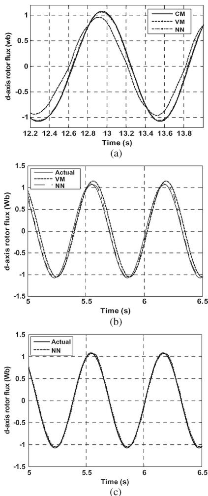
Fig. 4. NN observer testing. (a) LPF effect (experimental). (b)  $R_s$  25% variation (simulation). (c)  $R_r$  50% variation (simulation).
