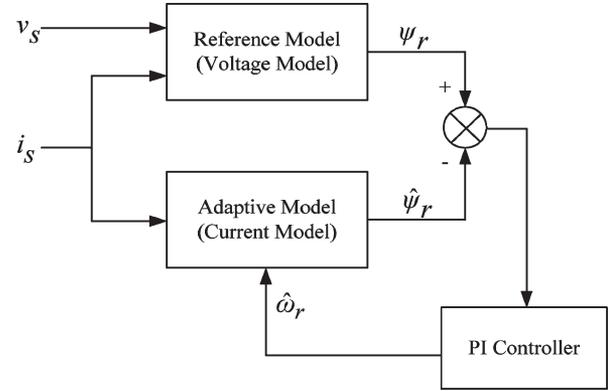
Fig. 1. Classical rotor flux MRAS speed observer.
