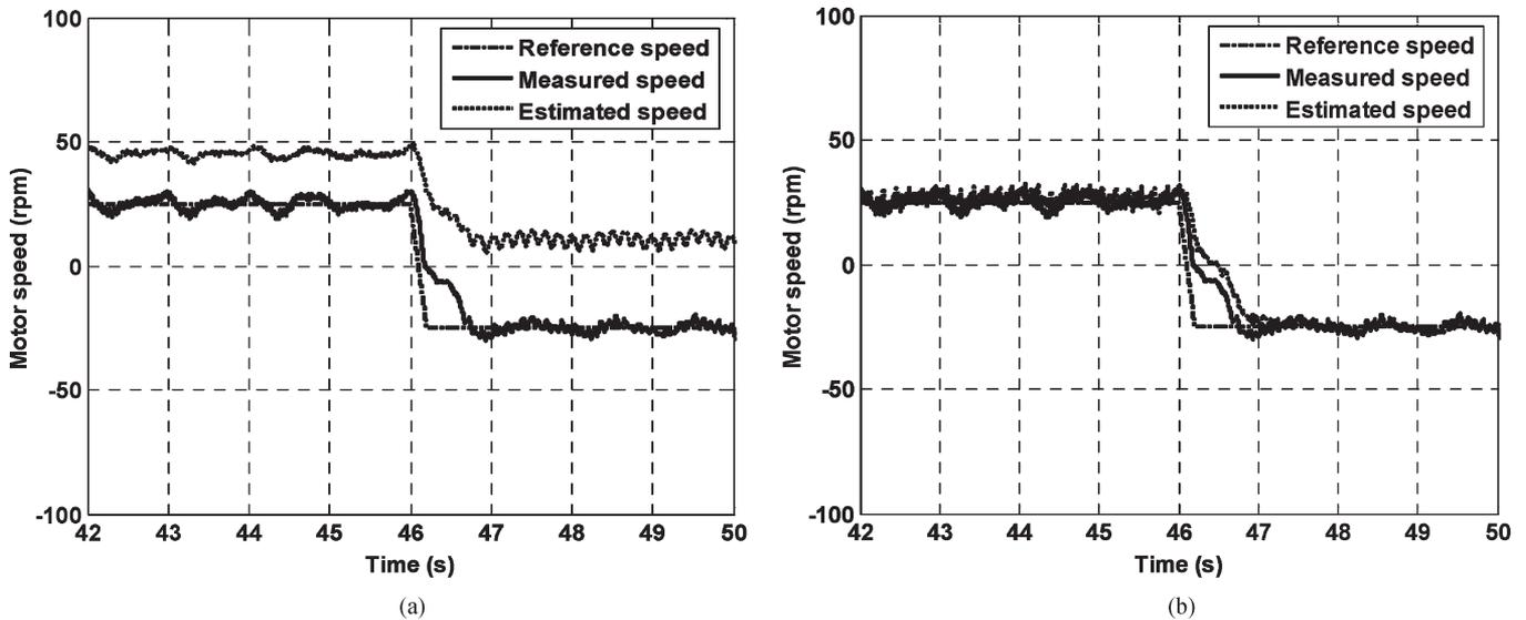
Fig. 7. Open-loop speed reversal from 25 to -25 r/min, at a rated load (100% load torque). Speed: (a) conventional MRAS. (b) NN MRAS.
