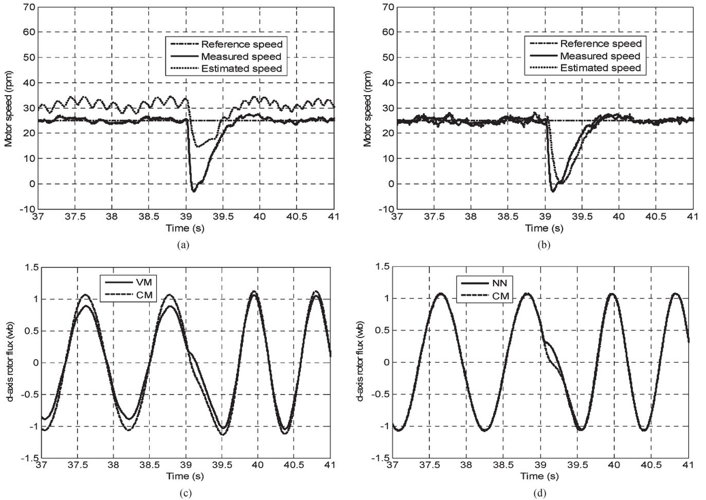
Fig. 6. Open-loop 20% load torque disturbance rejection, 25 r/min. Estimated speed: (a) conventional MRAS. (b) NN MRAS. Model outputs: (c) conventional MRAS. (d) NN MRAS.
