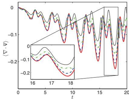
FIG. 2. (Color online) Compressibility of the particle velocity field  $\langle \nabla \cdot \bar{\mathbf{v}} \rangle$  in the synthetic flow ( $A=\pi$ ,  $\omega=1$ ) as a function of time for  $St=0.2$ , measured by the FLM ( $d\langle \ln|J| \rangle/dt$ ; red solid line), and by the MEF on three different grid resolutions:  $10 \times 10$  grid cells (thin solid black line),  $20 \times 20$  grid cells (dash-dotted green line), and  $60 \times 60$  grid cells (dashed blue line).
