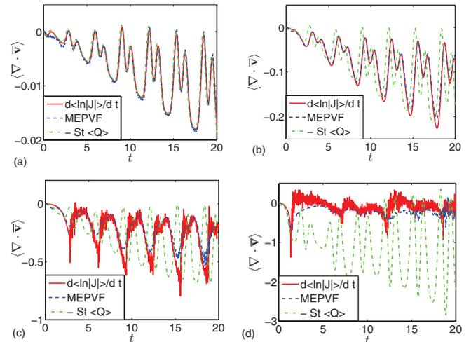
FIG. 1. (Color online) Compressibility of the particle velocity field  $\langle \nabla \cdot \bar{\mathbf{v}} \rangle$  in the synthetic flow ( $A = \pi$ ,  $\omega = 1$ ) as a function of time, measured by the FLM ( $d\langle \ln |J| \rangle / dt$ ; red solid line), and by the MEF (MEPVF; blue dashed line). Maxey's estimate, Eq. (3), is plotted as well (green dash-dotted line). (a)  $\text{St} = 0.05$ , (b)  $\text{St} = 0.2$ , (c)  $\text{St} = 0.5$ , and (d)  $\text{St} = 2$ .
