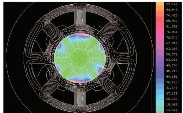
Fig. 5 Flux and loss contour plot produced for the 100kW machine using a time-stepping method.
