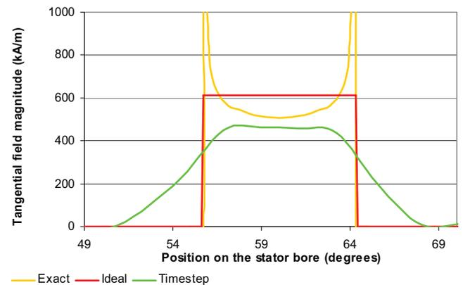
Fig. 10 Tangential field profile at the slot opening.
