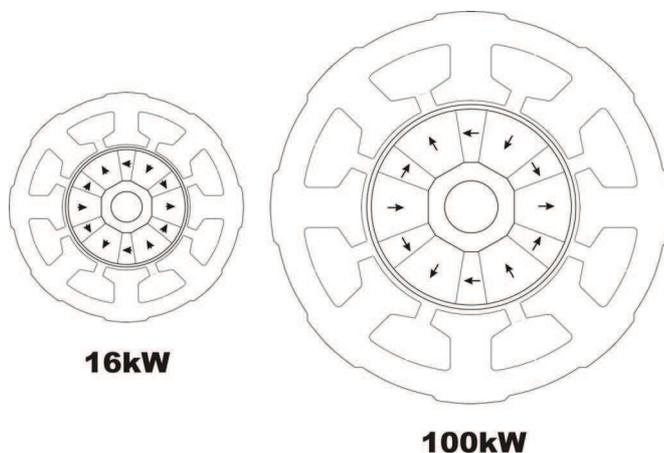
Fig. 2 Comparison between the 16kW and a 100kW fault tolerant motor
