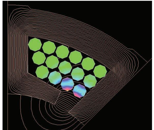
Fig. 4 2D-FE simulation of winding loss using the new stator design.
