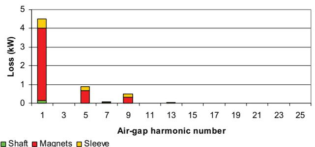
Fig. 8 Rotor eddy current loss spectrum
