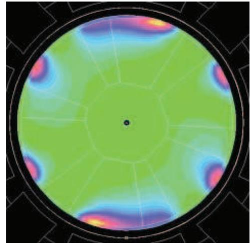
Fig. 9 Rotor eddy current shade plot.
