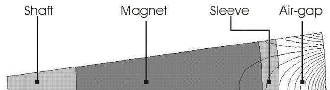
Fig. 7 2DFE model of the 15th harmonic applied to a section of the rotor
