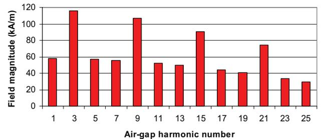
Fig. 6 Air-gap tangential magnetic field spectrum of the 100kW machine
