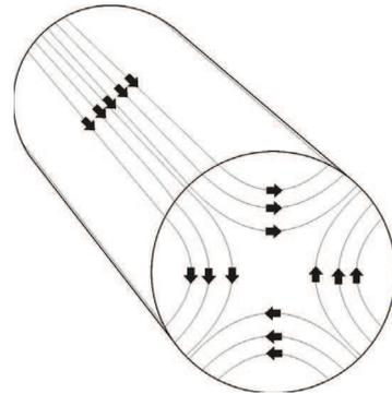
Fig. 13 Eddy current path in a solid rotor. [14]
