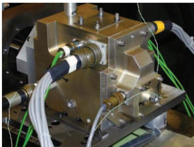
Fig. 1 16kW fault tolerant electric motor on test bed.
