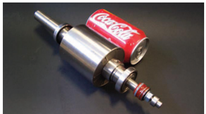
Figure 3. The 100kW permanent magnet rotor.
