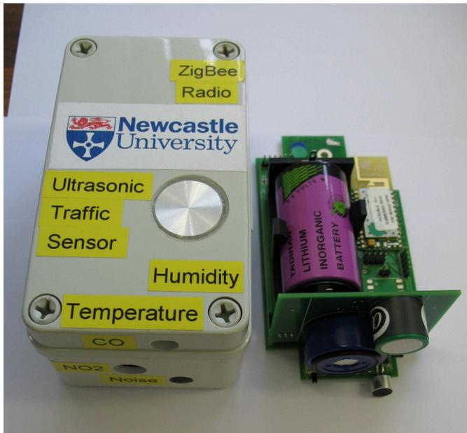
**Figure 2: MESSAGE Mote Packaging and Electronics**
