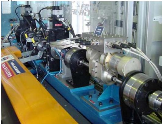
Figure 6: DEAWS flap actuator test rig.
