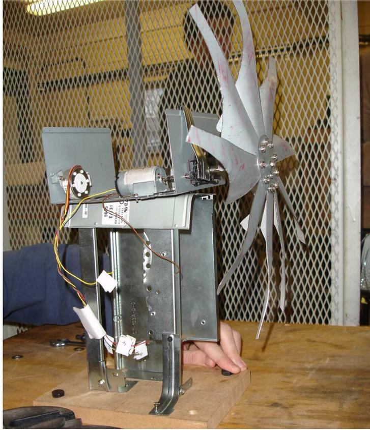
Figure 1: a wind turbine based on components and material from a redundant computer and printer
