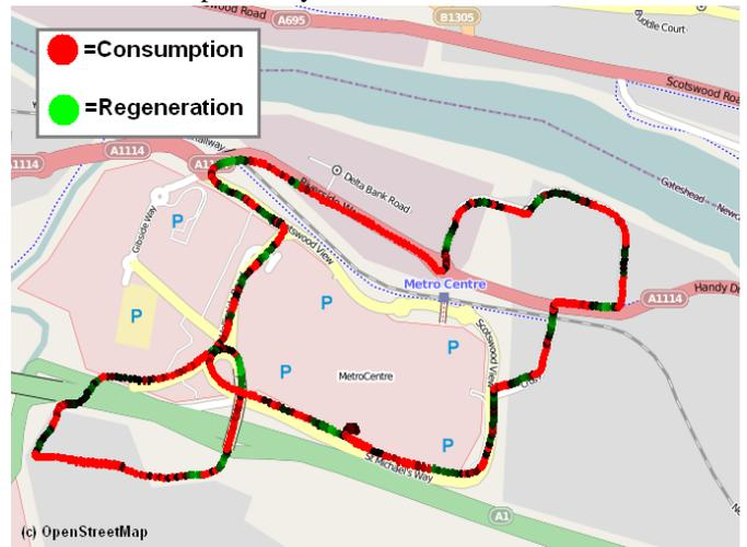
Figure 8 The basic pattern of consumption and regeneration over the course of a single journey can be seen here. It can be seen that the majority of distance is undertaken with consumption with only a small proportion using regeneration.
