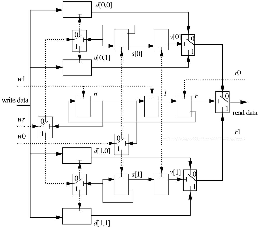
**Figure 3 Four-slot mechanism.**
