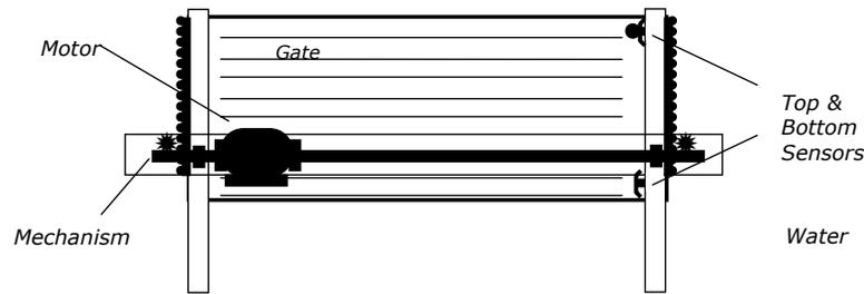
**Fig. 2.** A representation of a sluice gate
