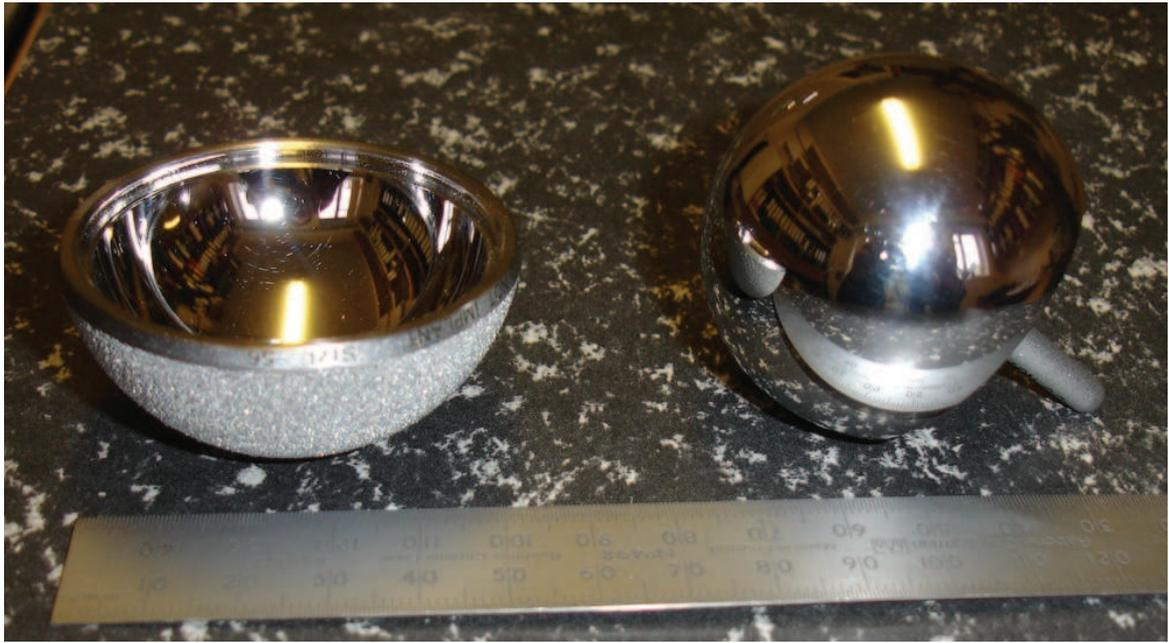
Figure 1: An unused ASR™ resurfacing hip prosthesis, acetabular cup to the left and femoral head to the right
