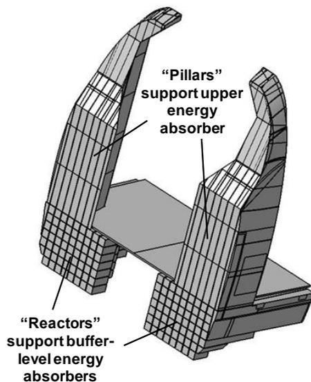
Figure 4 – D-CAB’s reinforced sandwich sections.
