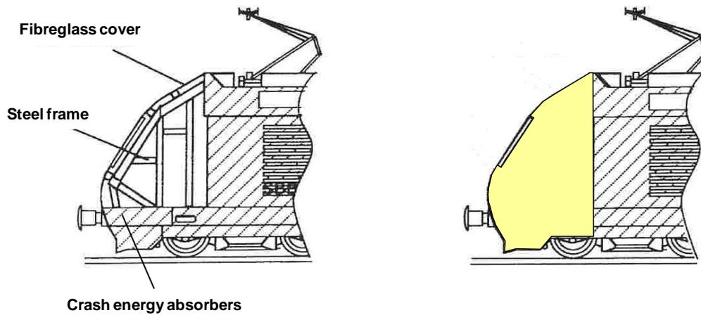
Figure 1 – the contrast between a conventional cab structure (left) with fragmented components and materials, and the highly integrated composite sandwich solution developed by the authors (right). The figure is a modified version of that presented by Cortesi et al. [2].
