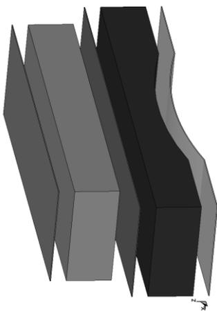
Figure 8 – the multi-layer aluminium honeycomb sandwich construction employed for D-CAB's upper energy absorber.
