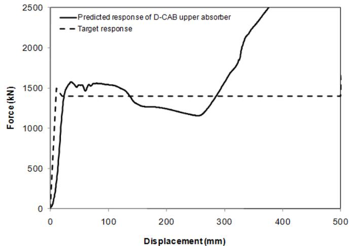
Figure 9 – a comparison between the predicted (solid line) and target (dotted line) load-displacement characteristics for the upper energy absorber.
