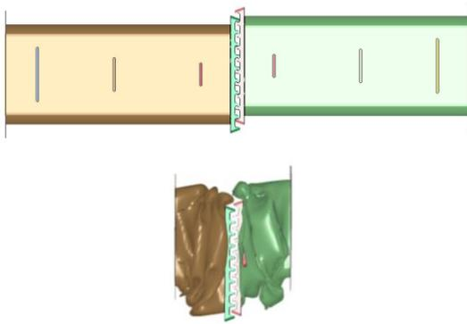
Figure 6 – the predicted collapse behaviour of two D-CAB buffer-level energy absorbers in a face-to-face collision.
