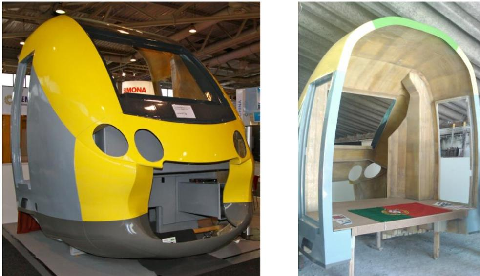
Figure 10 – the full-scale prototype of the lightweight crashworthy D-CAB concept.
