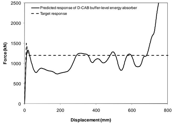
Figure 7 – a comparison between the predicted (solid line) and target (dotted line) load-displacement characteristics for a D-CAB buffer-level energy absorber.
