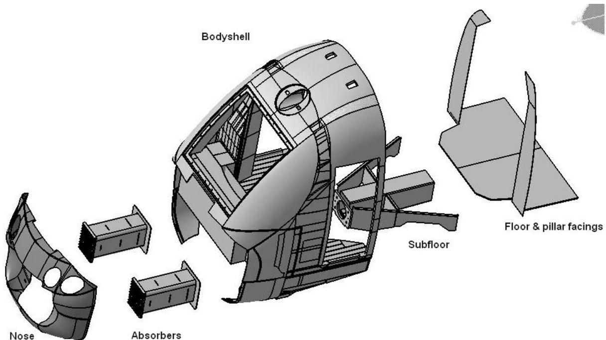
Figure 3 – an exploded view of the overall D-CAB design concept.
