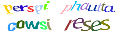
Figure 12. Segmentation results of the Google scheme: each segmented character is highlighted with a distinct color.
