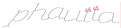
Figure 7. Detecting characters with a cross shape (the detected cross shapes are highlighted by a red box).
