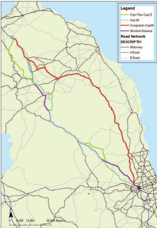
Figure 7: Routing to minimise energy consumption under different levels of network capacity.
