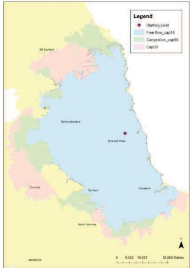
Figure 8: Driving range of an EV for different levels of network capacity.
