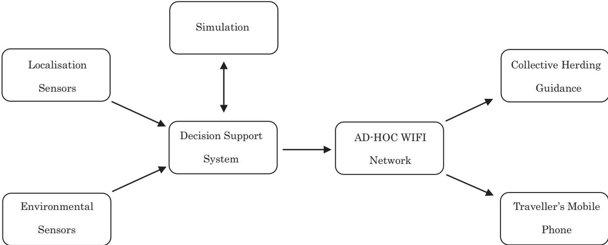
**Figure 1 - Simplified Architecture of SAVE ME System**
