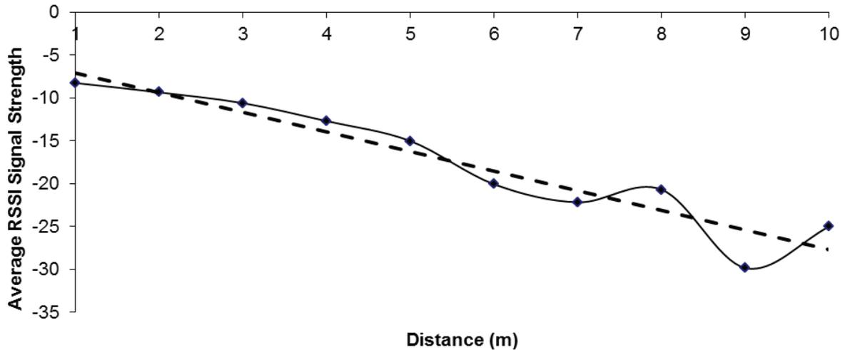
**Figure 3 – Average RSSI Signal Strength as a function of distance**
