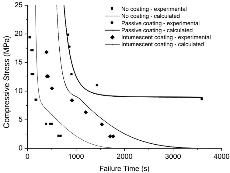
Figure 5. Effect of applied compression stress on the failure times of the laminate with or without fire protection coating. The data points show the experimental failure times and the curves were calculated using the model. The passive coating was 25 mm thick. The incident heat flux was  $50 \text{ kW/m}^2$ .
