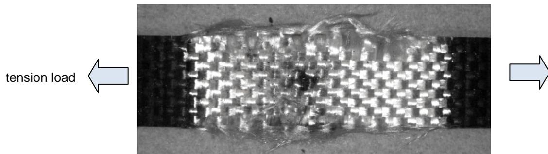
Figure 8. Tensile failure of the laminate during fire structural testing involved rupture of the load-bearing plies. The white region shows where the glass fibres have been exposed due to decomposition and vaporisation of the polymer matrix.
