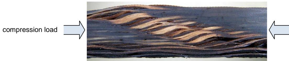
Figure 6. Compressive failure of the laminate during fire structural testing involved plastic microbuckling of the load-bearing plies and delamination cracking between the plies.
