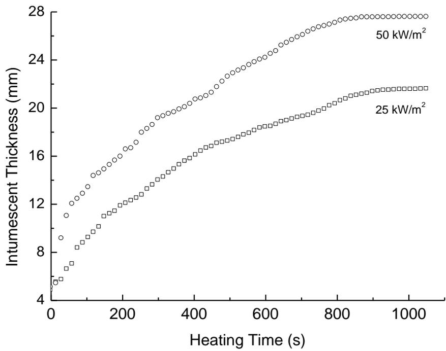
Figure 3. Effect of heating time on the thickness of the intumescent coating when exposed to the heat fluxes of 25 and 50 kW/m<sup>2</sup>.
