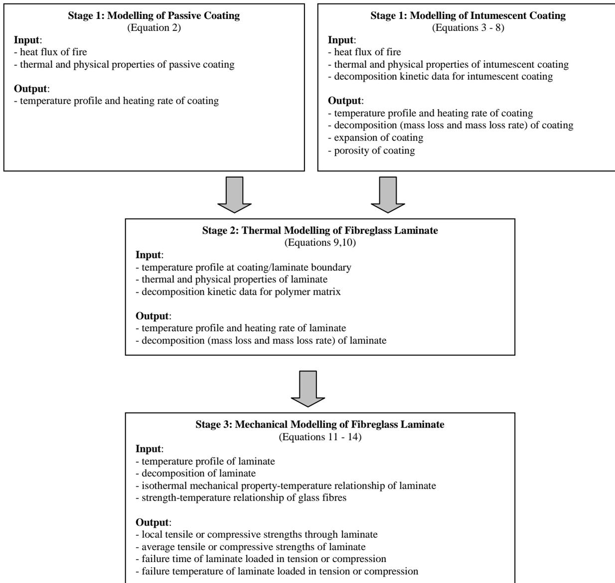
Figure 1. Summary flow-chart of the three-stage modelling approach to calculate the fire structural properties of fibreglass laminates with passive or intumescent insulation coating.
