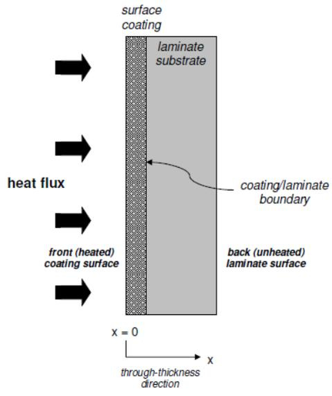
Figure 2. Representation of the laminate substrates protected with passive coating or intumescent coating.
