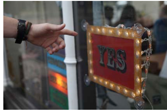
Figure 5. Lights illuminate the frames of the 'yes' and 'no' signs when the user's hand is detected in front of them
