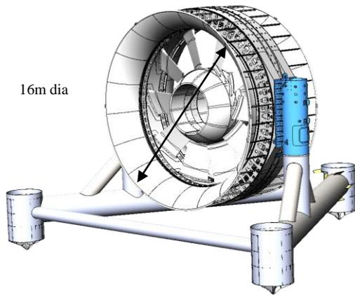
Figure 1: Open Hydro 16m commercial turbine
