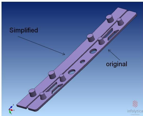
Figure 6: Example of mechanical component simplified for the purpose of meshing
