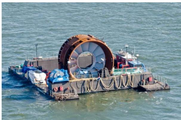
Figure 3: A 10m prototype on its deployment barge
