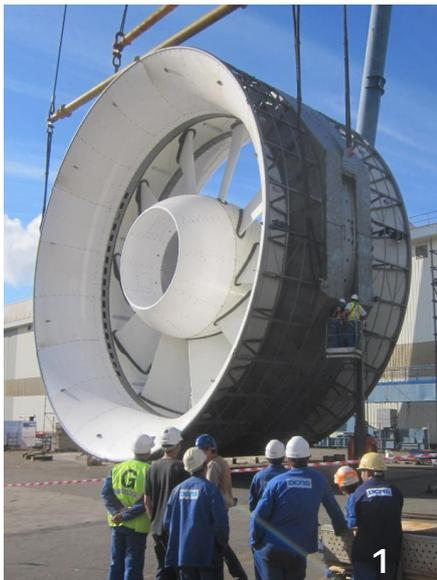
Figure 2: The 16m prototype during construction
