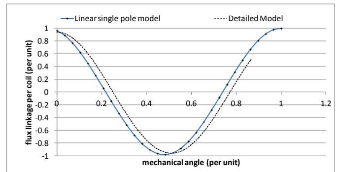
Figure 9: Comparison of flux linkage for full and single pole pair linear models.
