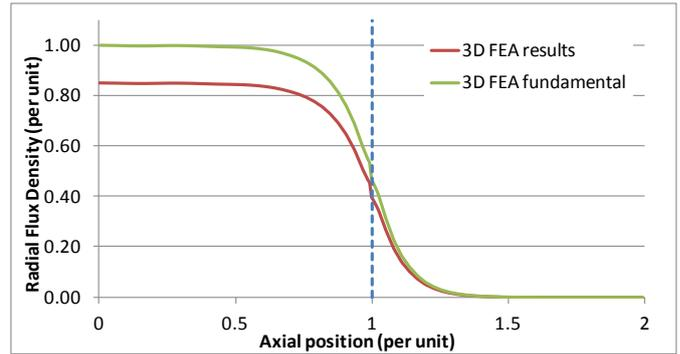
Figure 11: Axial variation of fundamental flux amplitude. The dotted line represents the edge of the magnet.
