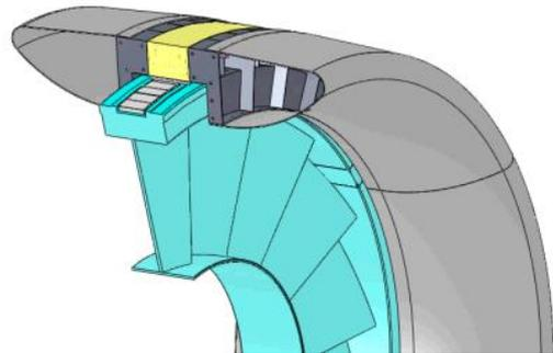
Figure 4: The arrangement of the PM rim generator
