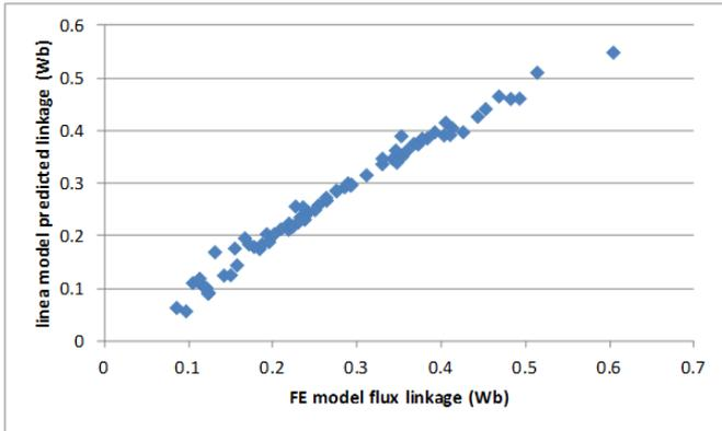
Figure 12: Plot of linkage predicted by linear equation verses FEA generated results.
