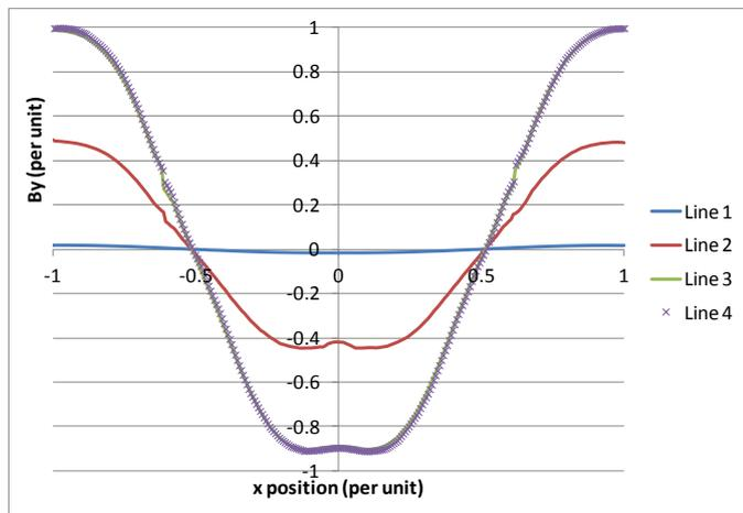
Figure 10: Radial flux density at the coil axis at the coil mean radius
