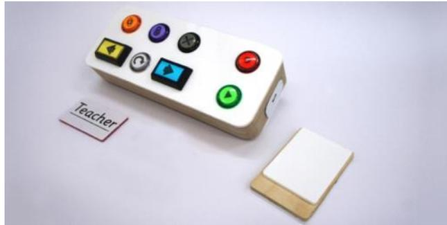
**Figure 4. Photo-sorting Console with RFID card & reader**
