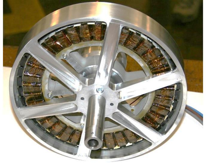
Fig. 1. Prototype motor with compressed aluminium windings.
