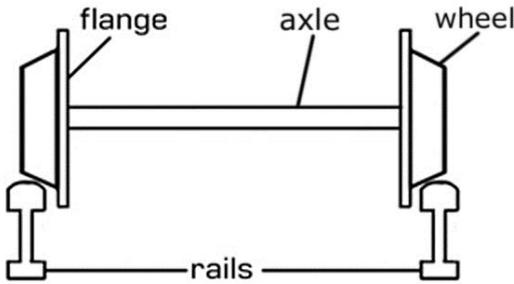
Figure 1: The Wheel Rail Interface.
