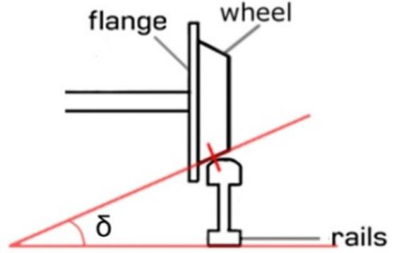
Figure 2: The Angle of Attack.
