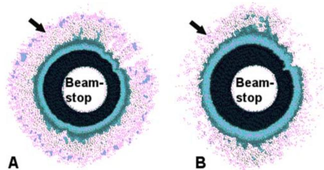
**Figure 4. Synchrotron X-ray diffraction patterns from amnion.** Representative (false colour) patterns collected from amnion proximal (a) and distal (b) to the placenta. Arrows indicate position of the interfibrillar reflection (magenta) other coloured rings close to the beamstop are background/backscatter. X-ray diffraction patterns displayed an anisotropic arrangement of collagen fibrils within the distal amniotic tissue. doi:10.1371/journal.pone.0001147.g004
