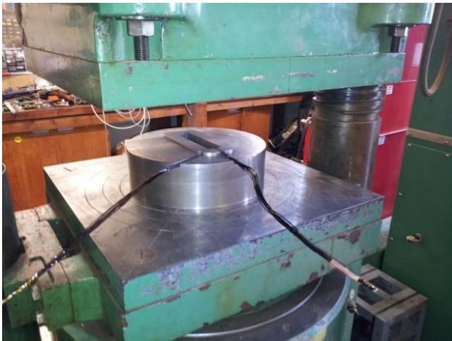
Fig. 8: Die tooling positioned in 500 tonne press ready for compression. Wire terminations are shown laid flat in specially prepared channels.
