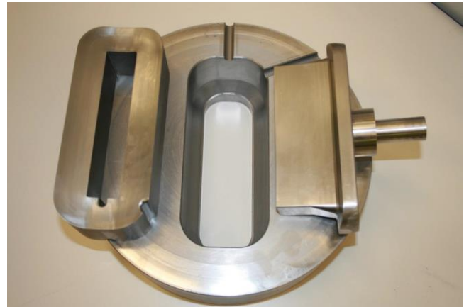
Fig. 6: Showing punch (left), die (bottom) and bobbin (right) set.
