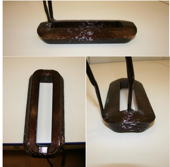
Fig. 9: Pre-Compressed Aluminum Motor coil with 77.9% gross fill factor following compression.
