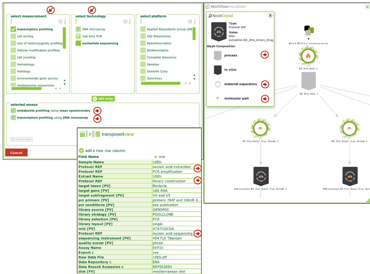
Fig 5. Panel (a) shows the assay selection panel in ISAcceptor (editor and curation tool) which uses OBI terms. Panel (b) shows ISA 'Protocol REF' elements, which are annotated with subclasses of 'OBI:planned process'. Panel (c) shows a glyph-based representation of the underlying mapping of ISA syntax element into OBI framework: circles correspond to Material or Data, which are 'specified_input_of' some 'OBI:planned process' either 'OBI: material transformation' or 'OBI:data transformation'. The graph matches by the underlying RDF representation.
