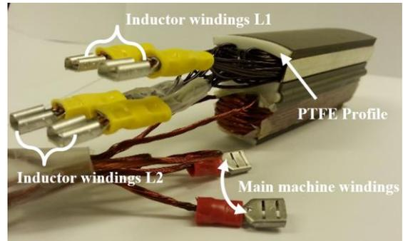
Fig. 11. 3D presentation of double slot tooth with end windings terminals
