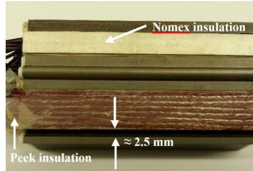
Fig. 10. On-tooth pressed coils
