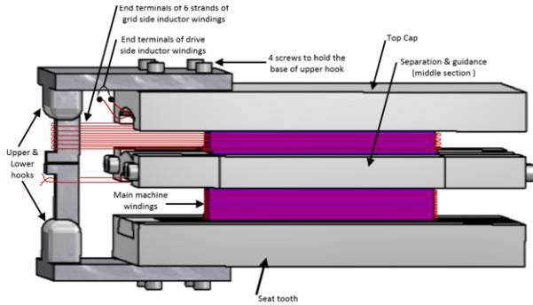
2. The winding jig is fitted to the tooth segment and the coils wound. Locating hooks hold the wire in place once wound
