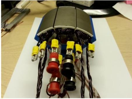
Fig. 13. Three tooth motorette with test leads
