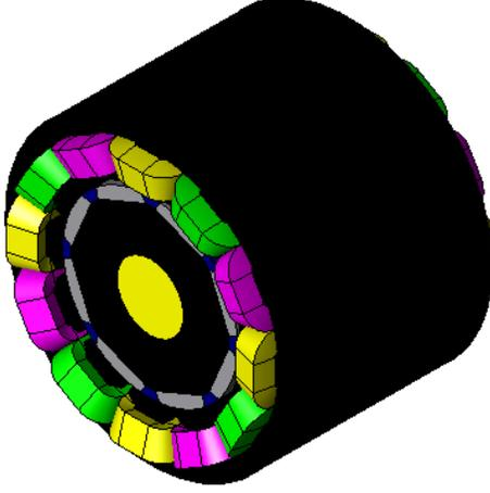
Fig. 2. 3D presentation of the high speed PMSM
