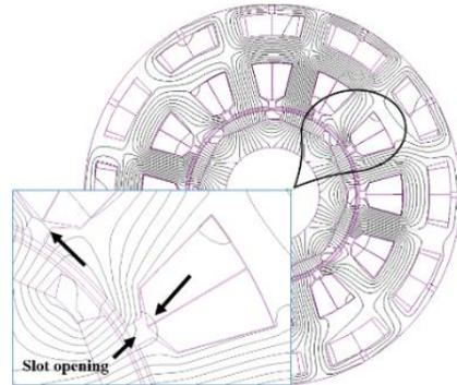
Fig. 8. Fringing in the slot opening
