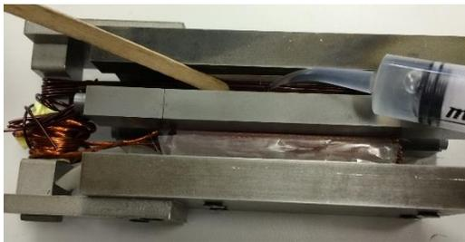
3. Coils are impregnated with thermally activated bonding agent, Ultimag 2002L.
