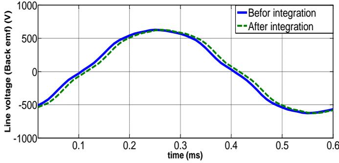
Fig. 6. The original machine back emf line voltage before and after integration
