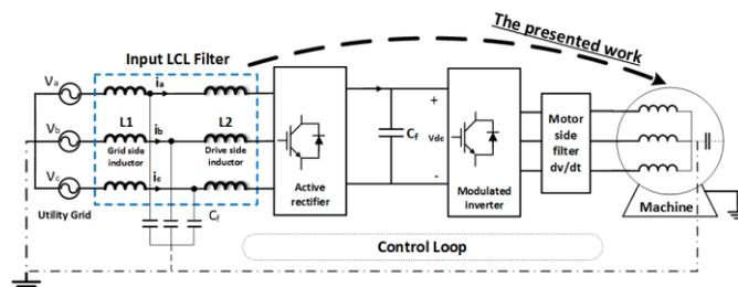
Fig. 1. A general schematic of an electric drive included input power LCL filter
