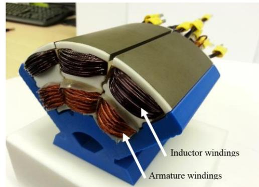
Fig. 12. 3-tooth fully assembled IDS motor
