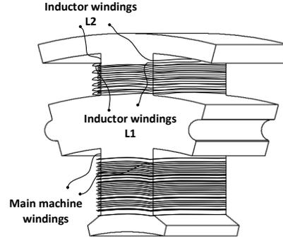
Fig. 7. Single tooth stator segment
