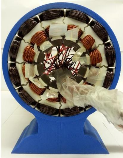
Fig. 14. The demonstrator of stator of integrated double slot machine
