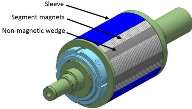
Fig. 3. Rotor assembly, showing segmented magnets
