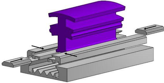
1. The stator tooth segment is loaded into the winding jig seat
