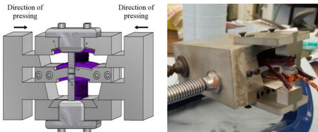
4. The pressing punch is applied and coils are forced into a regular shape. The assembly is placed in an oven at 165°C and the bonding agent is allowed to anneal.
