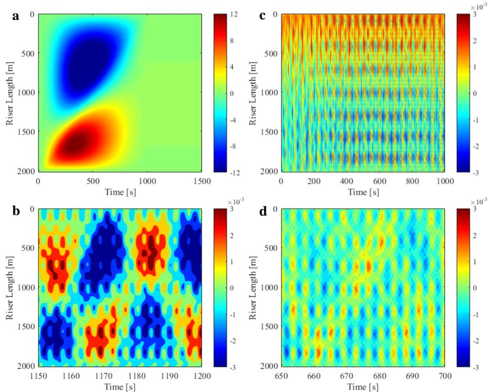
**Figure 5. Time-space varying normal response with 20D slug unit and equal gas and liquid lengths: a) transient displacements, b) magnified steady-state response, c) riser response after the transient by pre-locating the slugs, d) steady-state focus**
