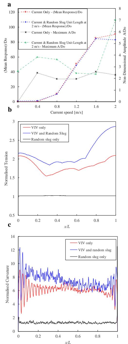
**Figure 12. a) Mean and maximum response for VIV only and VIV-SIV cases, with varying current flow speed, b) normalized maximum tension and c) curvature over the length of the riser in VIV and VIV-SIV cases**
