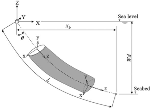
**Figure 1. Element model of steel catenary riser**
