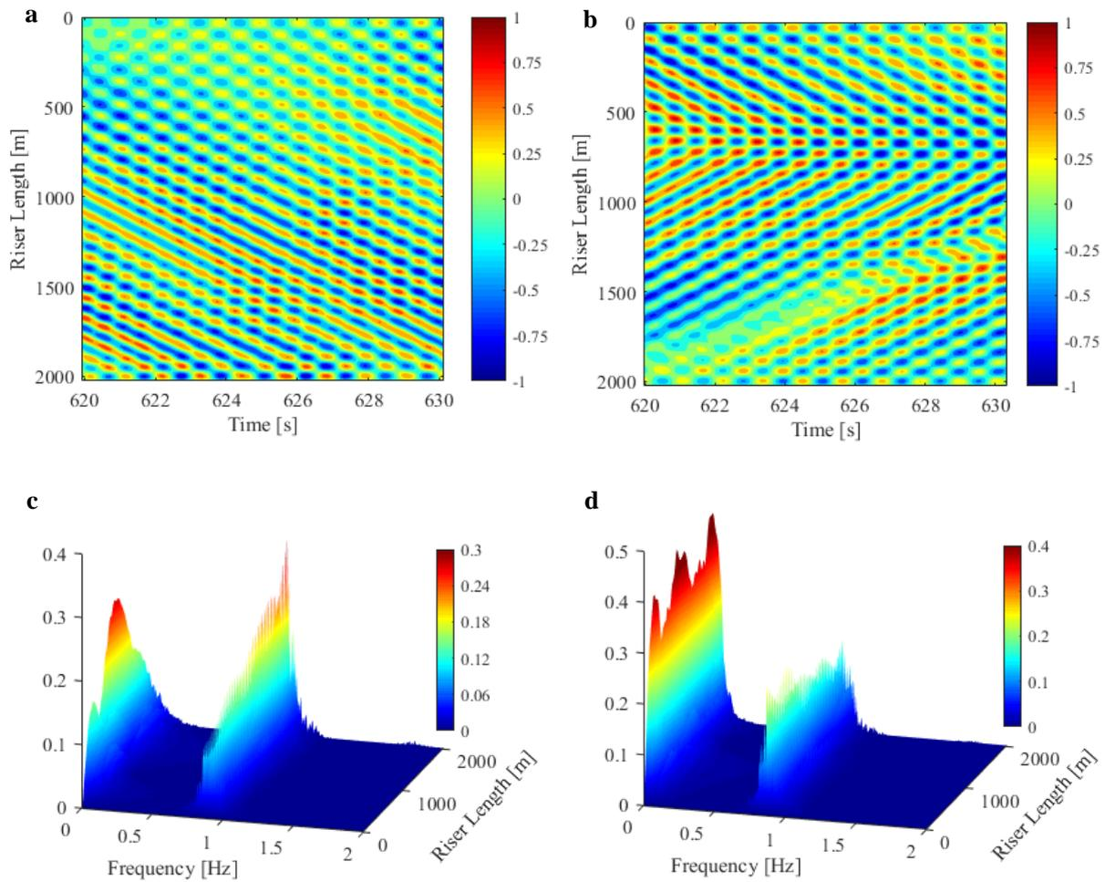
**Figure 10. a) Cross-flow time-space varying riser response with 2 m/s current flow involving b) random-length slug unit and liquid; frequency domain of c) VIV-only case and d) combined VIV-SIV with the non-uniform slug length**
