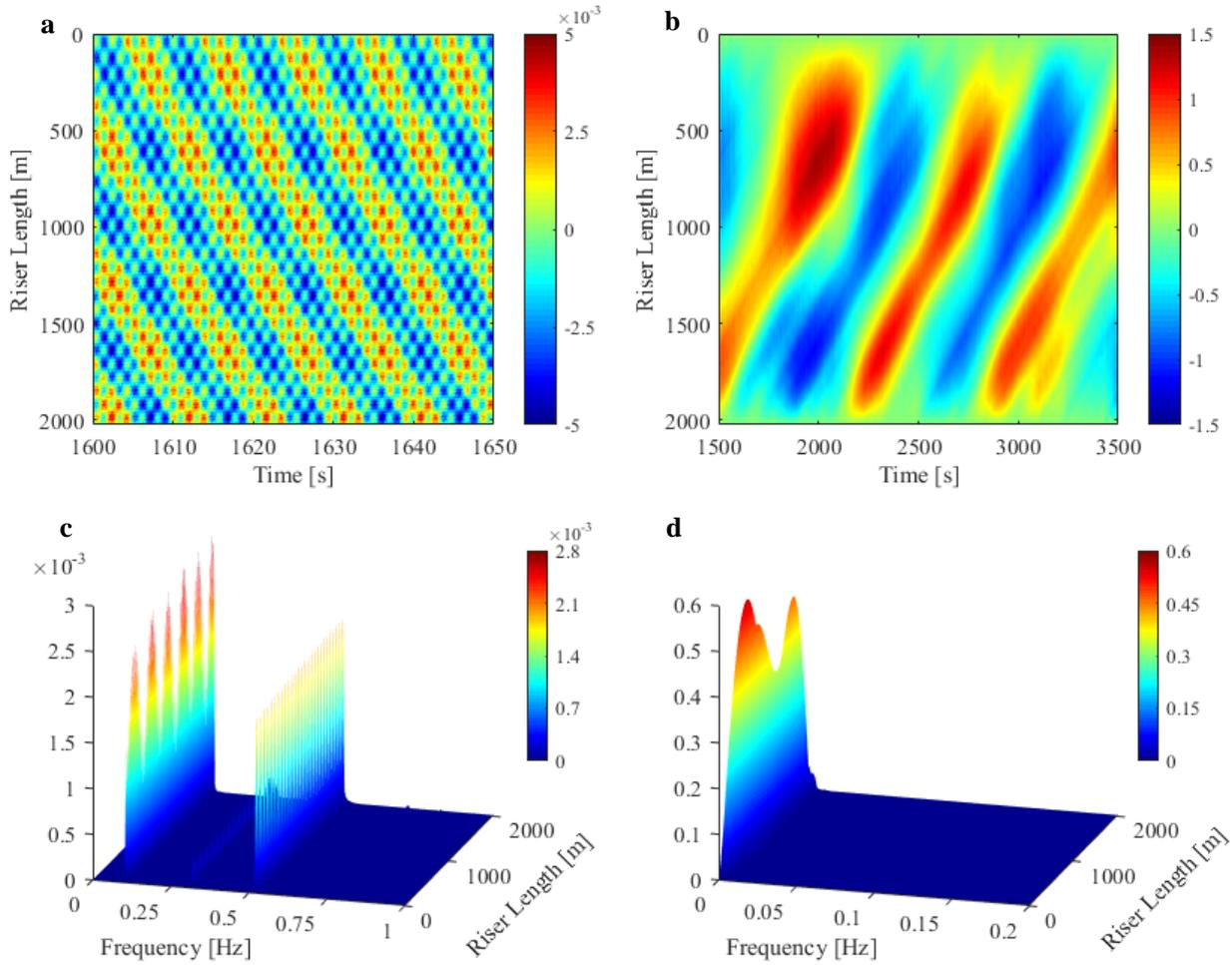
**Figure 9. Time-space varying response of catenary riser with a) uniform 50D slug unit with equal liquid and gas lengths, b) random slug unit and liquid lengths; the response frequency domain of c) uniform and d) non-uniform slug length cases**
