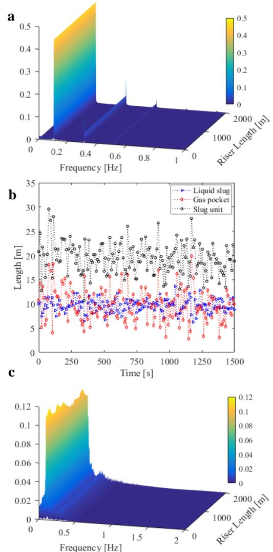
**Figure 8. Frequency domain plot of riser response with a) 50D slug unit with equal liquid and gas lengths, b) pseudo-random slug unit length and slug lengths, c) the corresponding frequency domain plot for random slug unit and liquid lengths**
