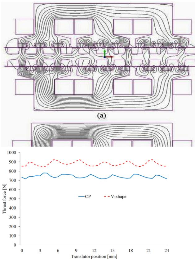
Figure10 Thrust force waveforms for both designs
