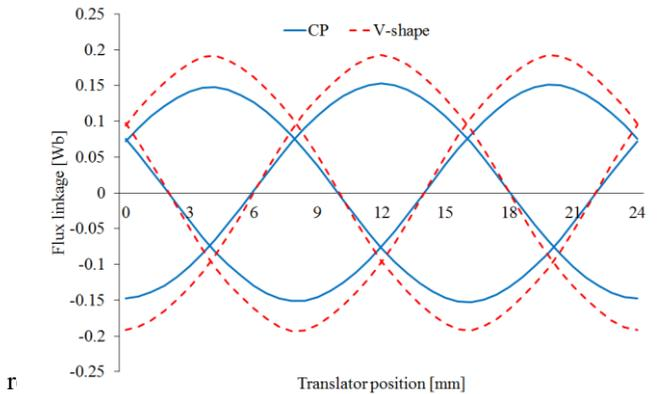
Fig.8 No-load flux linkage waveforms for both designs
