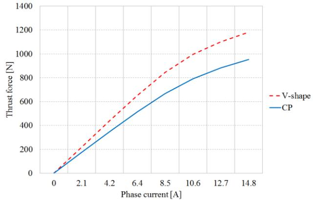
Fig.11 Overloading force capability for both machines
