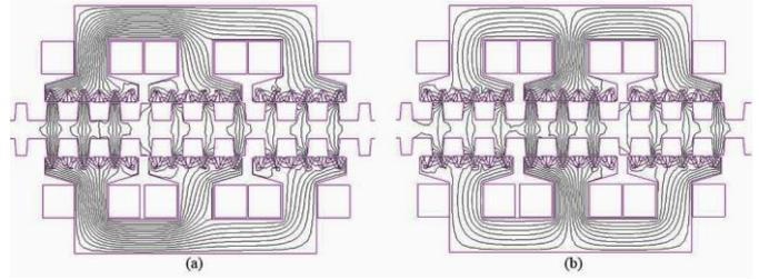
Fig.2 No-load field distribution (a)  $x=0$ , (b)  $x= 1/3\tau_1$
