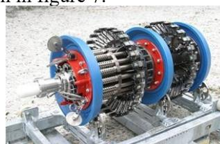
Fig 7. EC detector of ROSEN
