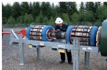
Fig 6. Rosen RoDD EMAT detector
