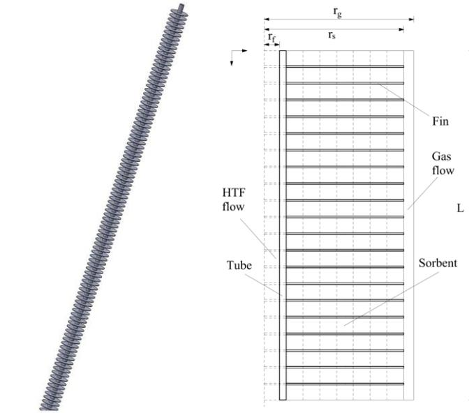
**Figure 3 Physical model of ammonia chemisorption modular finned-tube heat exchanger.**
