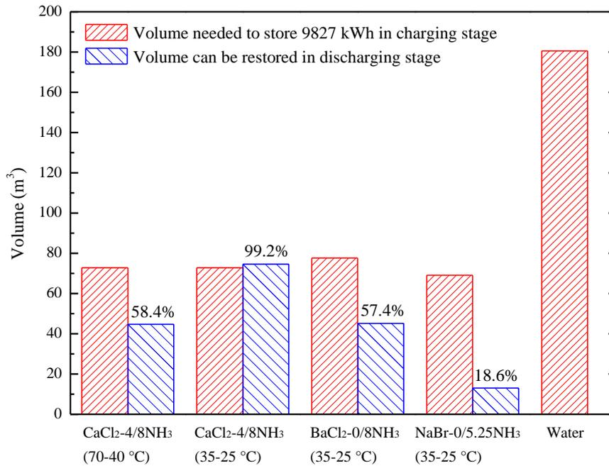
**Figure 8 Comparison between SSTES volume needed to storage 9827 kWh in charging stage and volume can be restored in discharging stage, volume of water system was calculated based on 54.4 kWh/m<sup>3</sup> storage density considering 25% heat loss [3, 6].**
