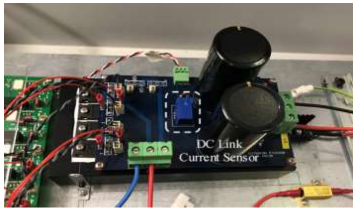
Fig. 9. H-bridge inverter with dc link current sensor
