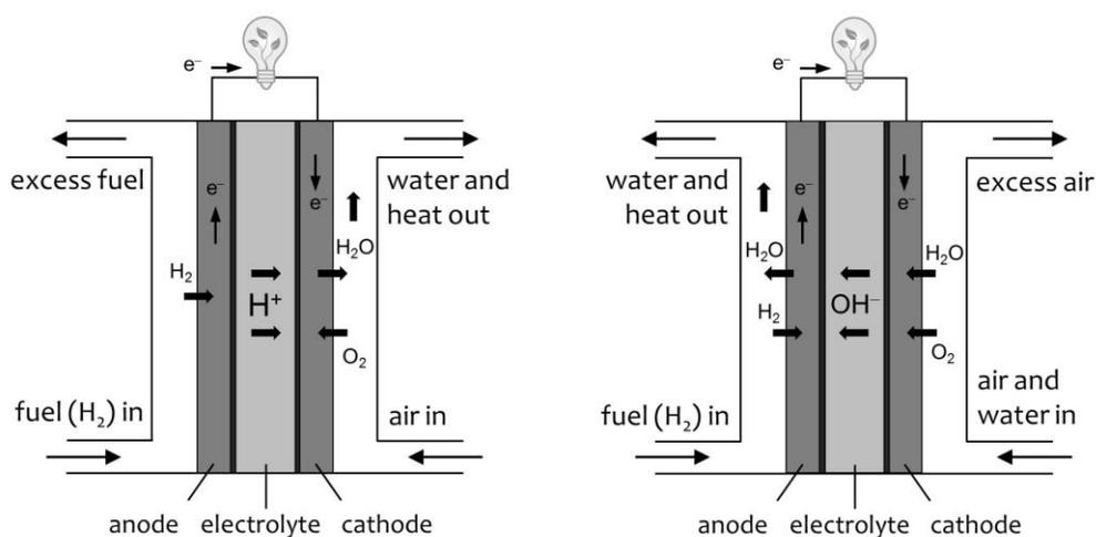
**Figure 16.2 – Schematic illustrations of a proton-exchange-membrane fuel cell (left) and an anion-exchange-membrane fuel cell (right).**
