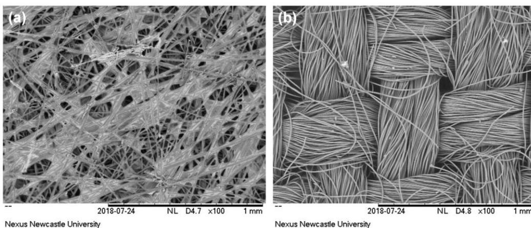
**Figure 16.6 – Scanning electron micrographs of typical (a) carbon paper GDL and (b) carbon cloth GDL.**
