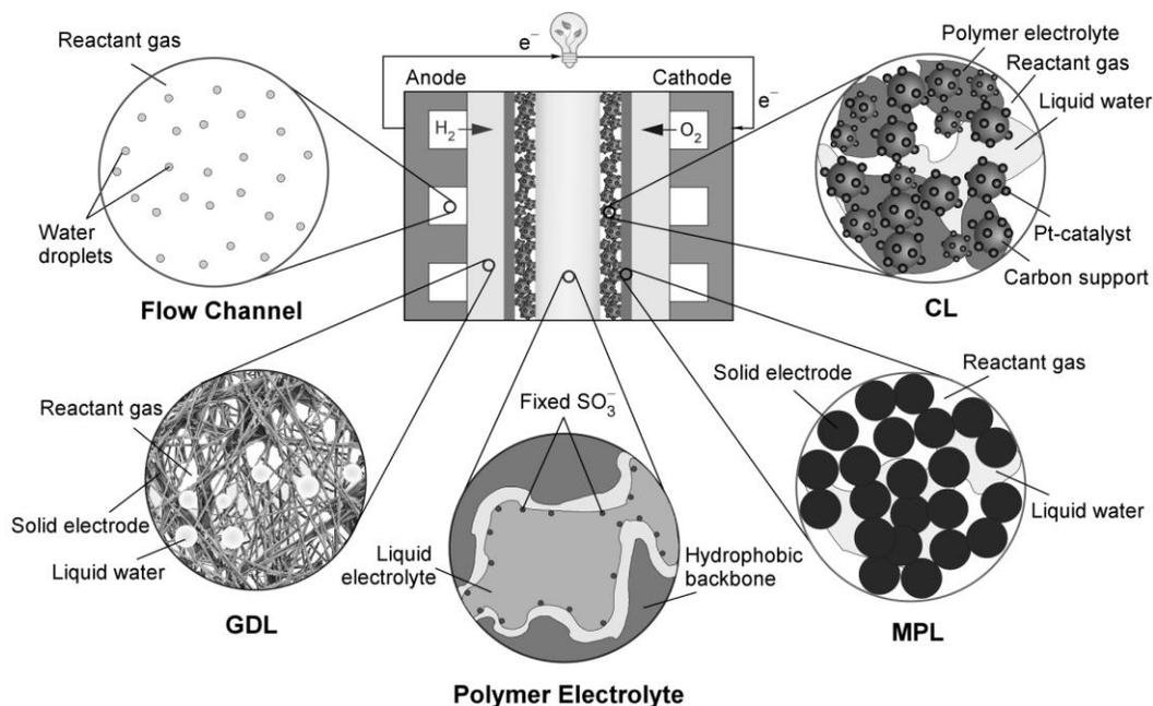
**Figure 16.4 – Physical structures of various layers of a PEFC.**
