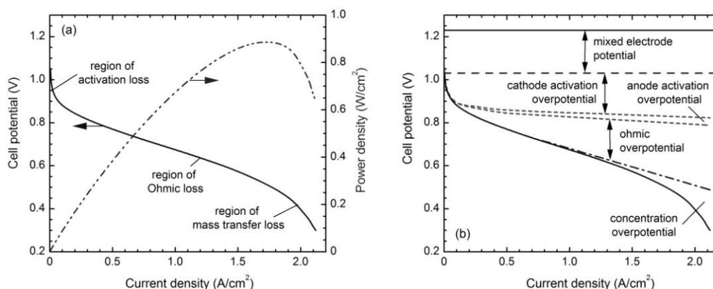
**Figure 16.3 – (a) A typical polarization and power density curves for PEMFCs with the region showing three main losses and (b) a breakdown of various overpotentials.**
