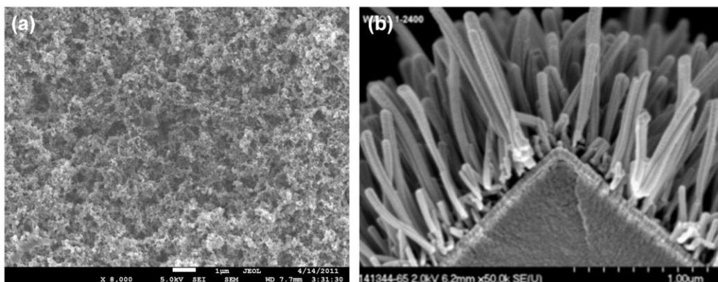
**Figure 16.5 – Scanning electron micrographs of (a) conventional Pt/C catalyst layer and (b) NSTF (PtCoMn alloy) catalyst layer (Das and Weber 2013, Debe 2012).**
