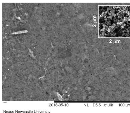
**Figure 16.7 – Scanning electron micrograph of a typical microporous layer.**
