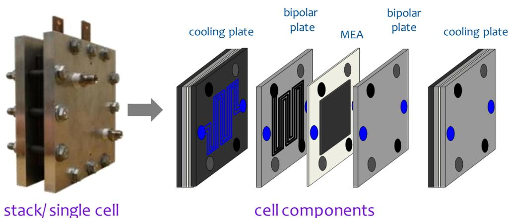
**Figure 16.1 – Images of a PEFC stack and single-cell and the schematic of various cell components (image sources: [www.fuelcellstore.com](http://www.fuelcellstore.com) and EnSys research group, [www.staff.ncl.ac.uk/prodip.das](http://www.staff.ncl.ac.uk/prodip.das)).**
