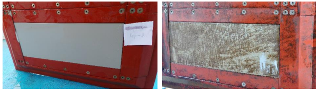
Figure 4 Test panels in clean and fouled conditions
