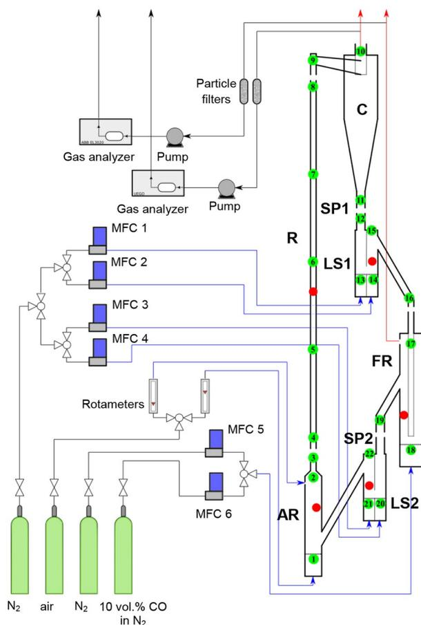
**Figure 3.** Schematic diagram of the experimental setup by using the CFB. AR: air reactor, C: cyclone, FR: fuel reactor, LS1: upper loop seal, LS2: lower loop seal, R: riser, SP1: upper standpipe, SP2: lower standpipe, and MFC: mass flow controller. The red circles indicate thermocouples. The green circles indicate the location of the pressure tappings (PT). The blue arrows represent the gas inlets, and the red arrows represent the gas outlets.
