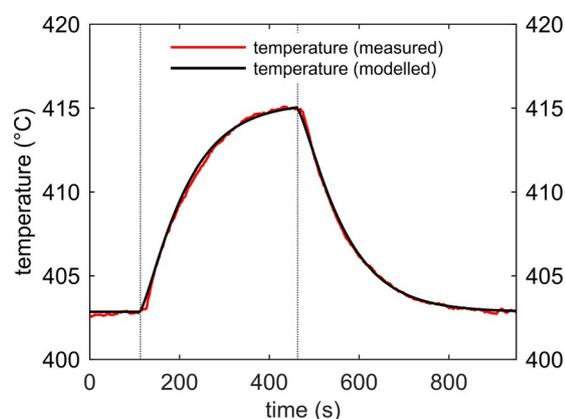
**Figure 1.** Temperature in the FR as a function of time, following the initiation of the reduction of the OC particles by CO. The red line corresponds to the measured temperature. The black line was computed by using Equation (11) with  $N=1.4$ ,  $k=0.75 \text{ WK}^{-1}$ ,  $Q_{\text{loss}}=160 \text{ JK}^{-1}$ , and  $t'_m=108 \text{ s}$ . The reactive gas was turned on for a total of 350 s, indicated by the vertical dashed lines.
