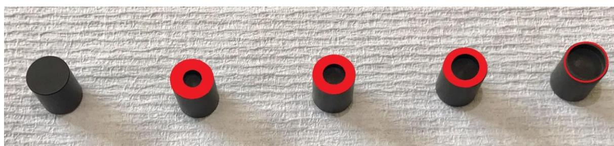
Figure 2 CFR PEEK test pins. From left to right, pin from group 1 (1.11 MPa), group 2 (1.38 MPa), group 3 (1.61 MPa), group 4 (2.00 MPa) and group 5 (5.30 MPa). Red circles were drawn for better contrast of the annulus.
