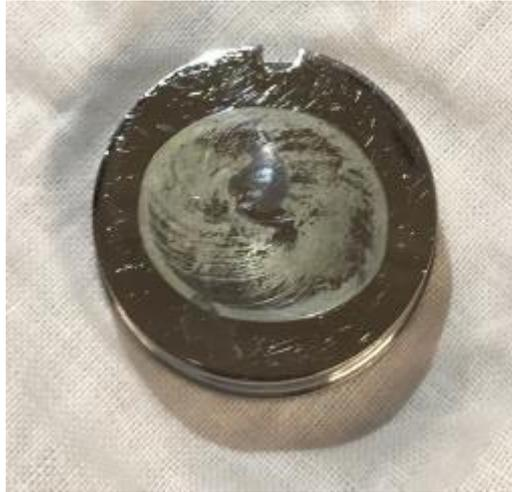
*Figure 9 A sample worn test disc after 2.5 million cycles of testing showing a central oval worn area.*
