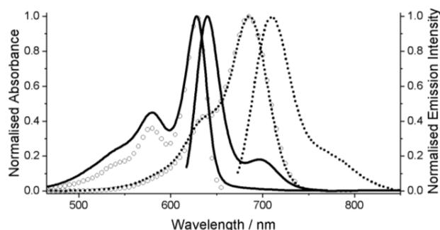
**Figure 2.** Room-temperature normalised UV/Vis-NIR absorption and emission spectra for compounds **BD** (solid line) and **CD** (dotted line) in cyclohexane. Excitation spectra are shown with open circles.
