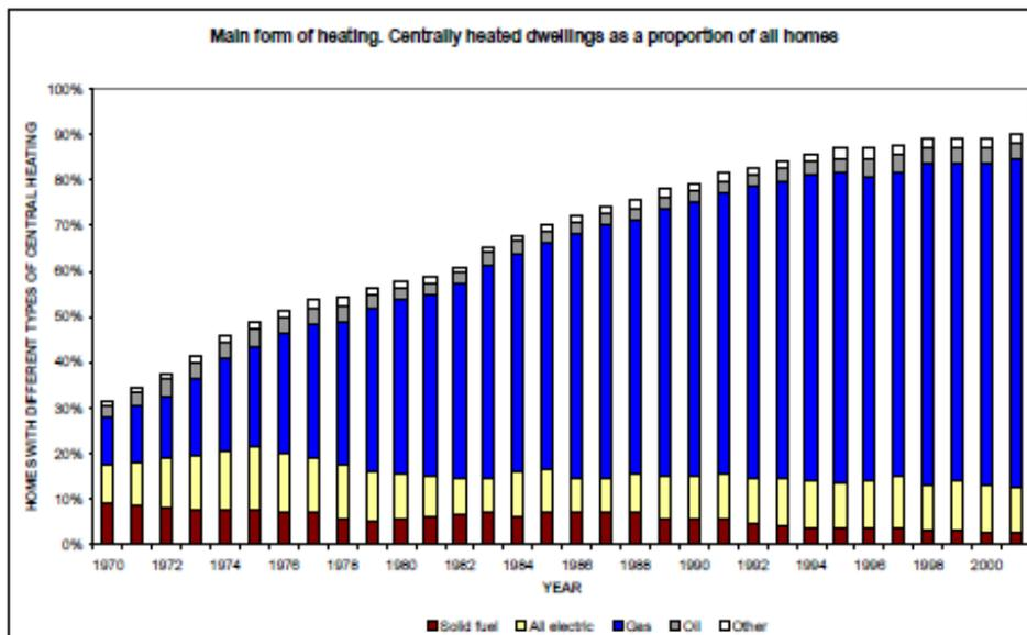
Figure 2 Main form of heating
