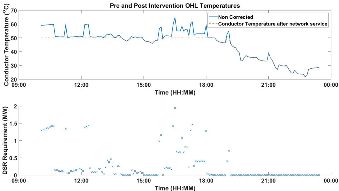
Figure 3 – Example of a maintaining the OHL circuit temperature limit through the use of DSR
