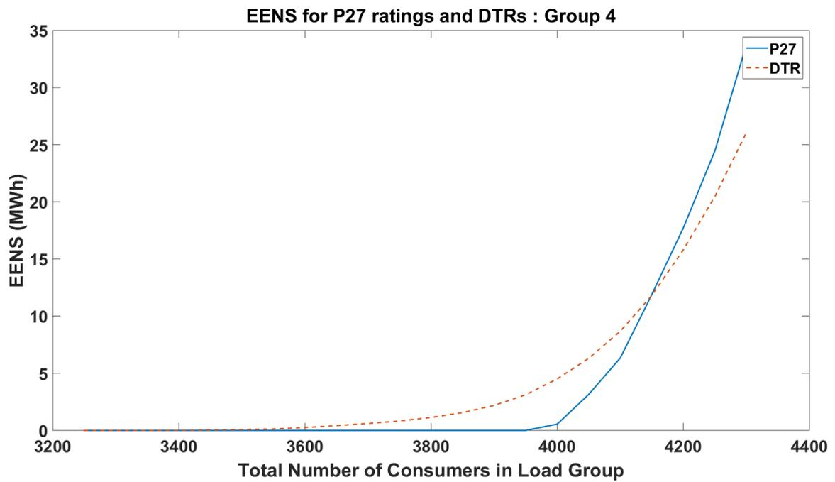
Figure 6 – EENS for Group 4 Loads at the case study location using both DTR and the presently implemented OHL ratings
