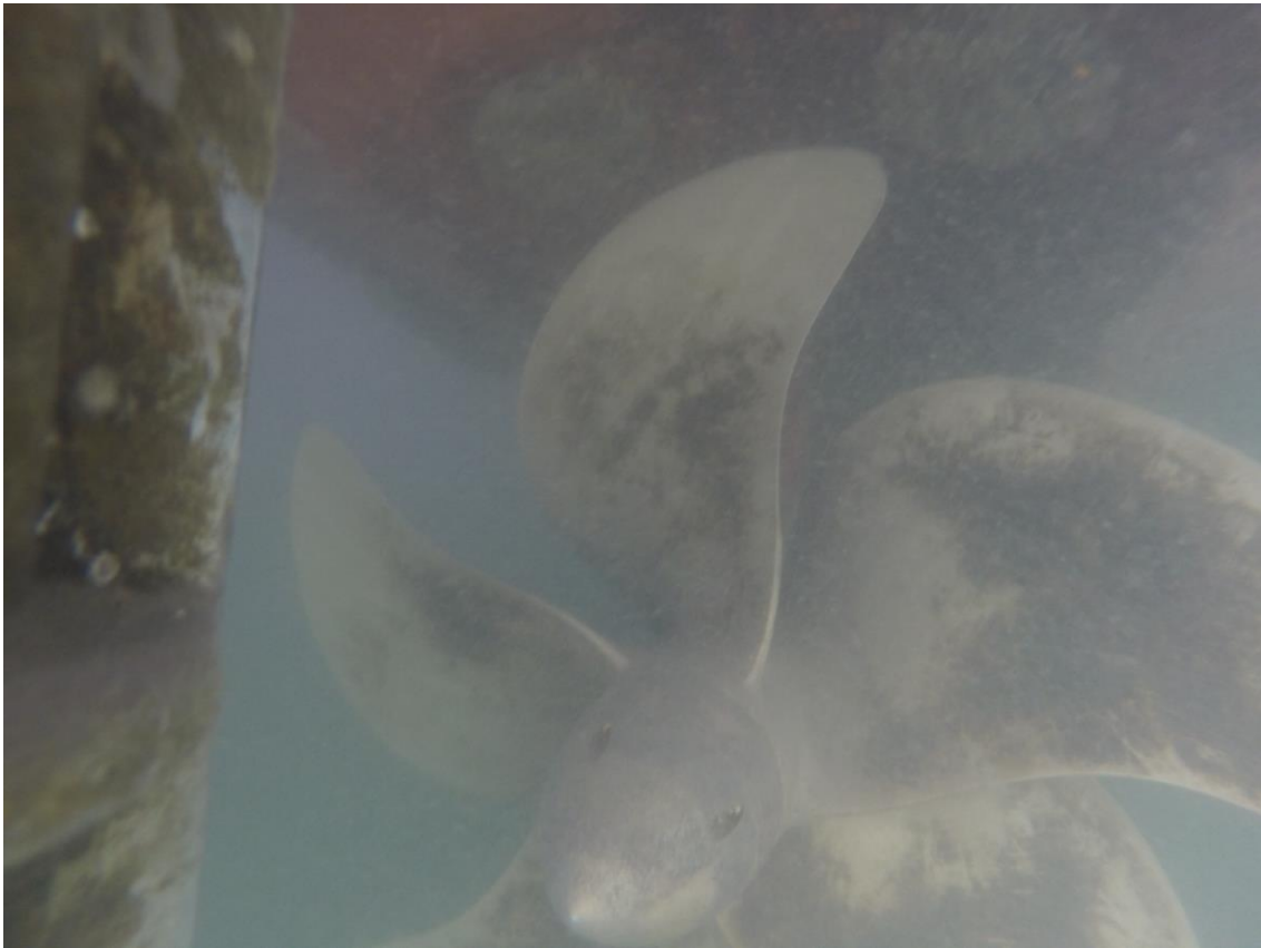
Figure B.4. Port propeller fouling photographed during an underwater survey in July 2018.
