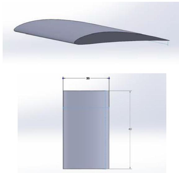
**Figure 11.** NACA 6412 with extrusion for the wing sail design (top), Wingsail design with dimensions (bottom).
