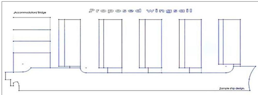
**Figure 12.** An artist's impression of the selected Oil Tanker with installation of 5 proposed wingsails.
