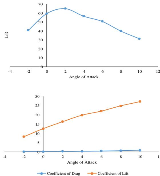
**Figure 9.** L/D vs angle of attack (top), Coefficient of lift and drag vs angle of attack (bottom).
