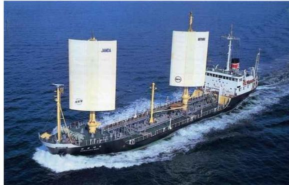
**Figure 3.** Shin-Aitoku Maru fitted with wingsails [6].
