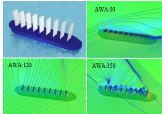
**Figure 6.** CFD simulations of modelled ship with wingsails at varying AWA [6].
