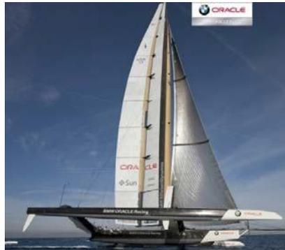
**Figure 1.** USA-17A racing boat with a rigid mainsail wingsail, and a conventional jib at the fore (source: Oracle team USA).
