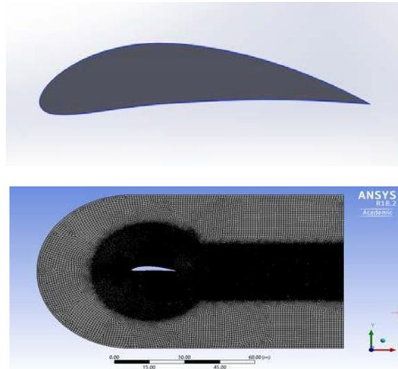
**Figure 8.** NACA 6412 modelled for simulation (top), Meshing in ANSYS Fluent for the aerofoil NACA 6412 (bottom).
