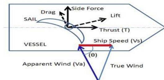
**Figure 2.** Forces acting on a wingsail [5].
