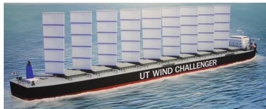
**Figure 4.** Artist impression of the UT challenger vessel with the installation of rigid, retractable wing sails [5].
