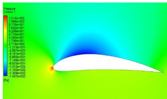
**Figure 10.** Pressure contour on NACA 6412 at maximum L/D at an angle of attack of 2°.
