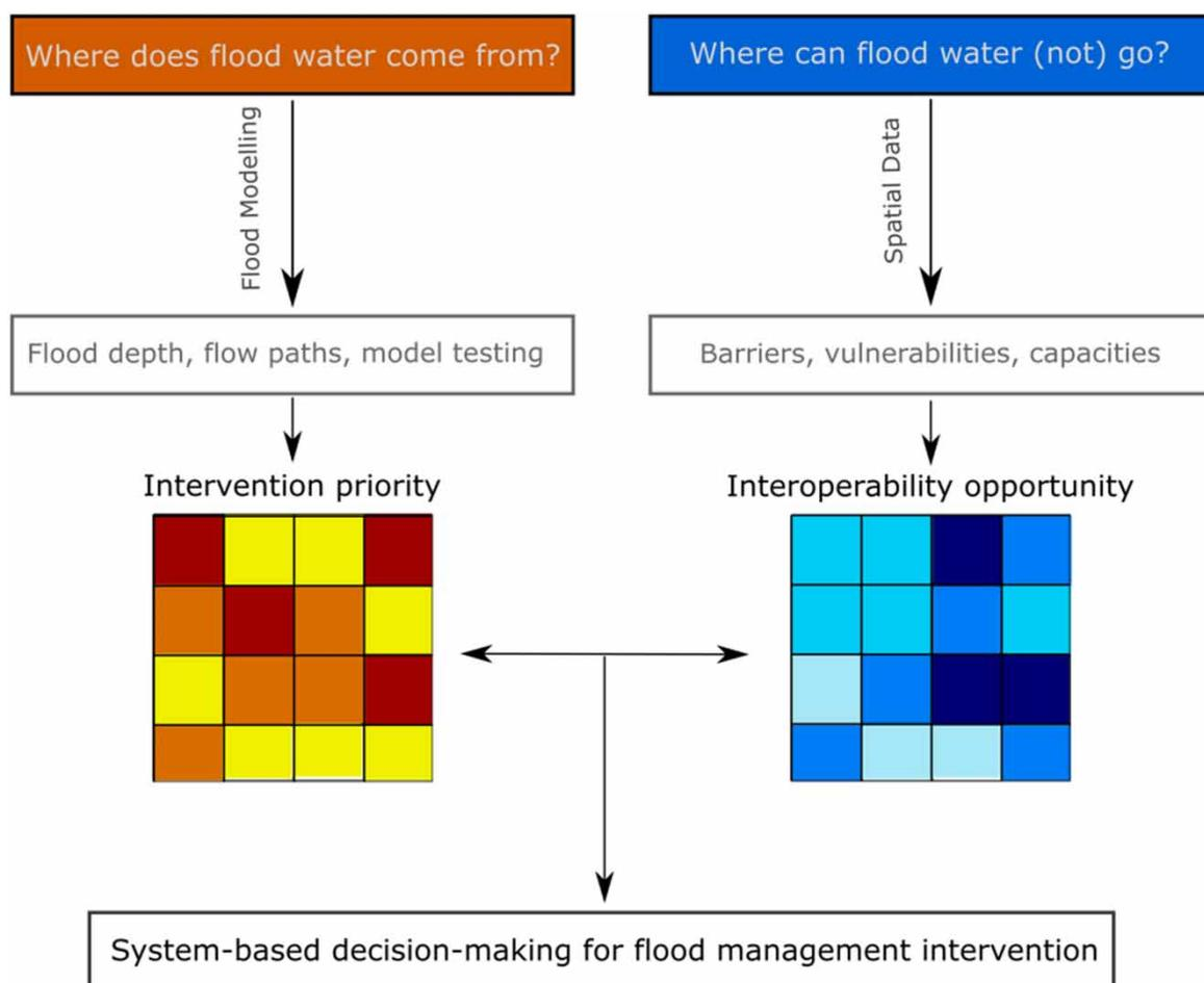
**Figure 8** | Conceptual architecture of a spatial mapping tool for system-based flood management aiming to combine two main aspects: (i) where does flood water come from and how can intervention priority areas be identified, and (ii) where can flood water (not) go based on the existing infrastructure systems that create opportunities and barriers for interoperability (Ver-cruysse *et al.* 2019).
