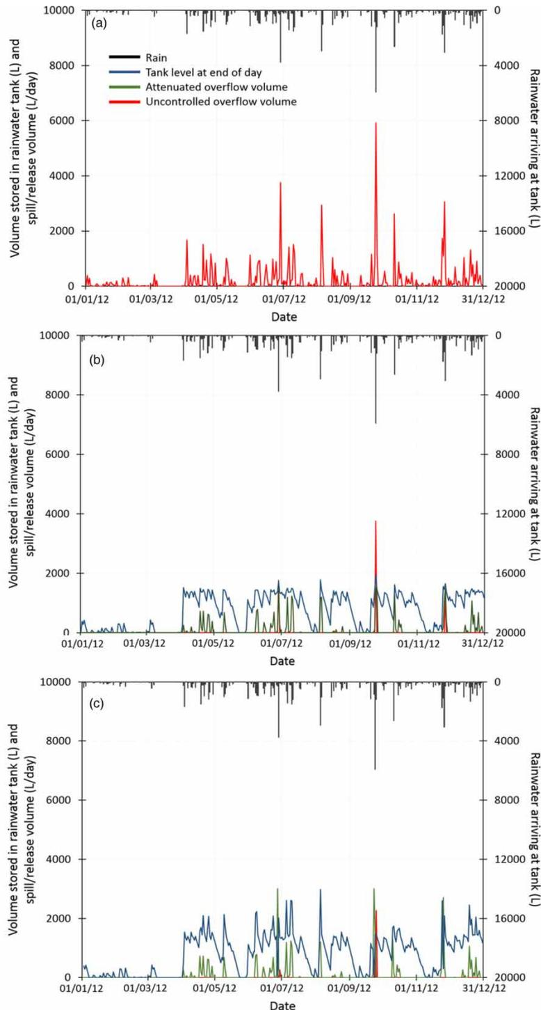
**Figure 6** | Household stormwater management based on a 3-bedroom house in Newcastle with an 80 m<sup>2</sup> roof area, using Newcastle rainfall data from 2012. (a) Without RMS (Rainwater Management System), (b) passive RMS and (c) active RMS.
