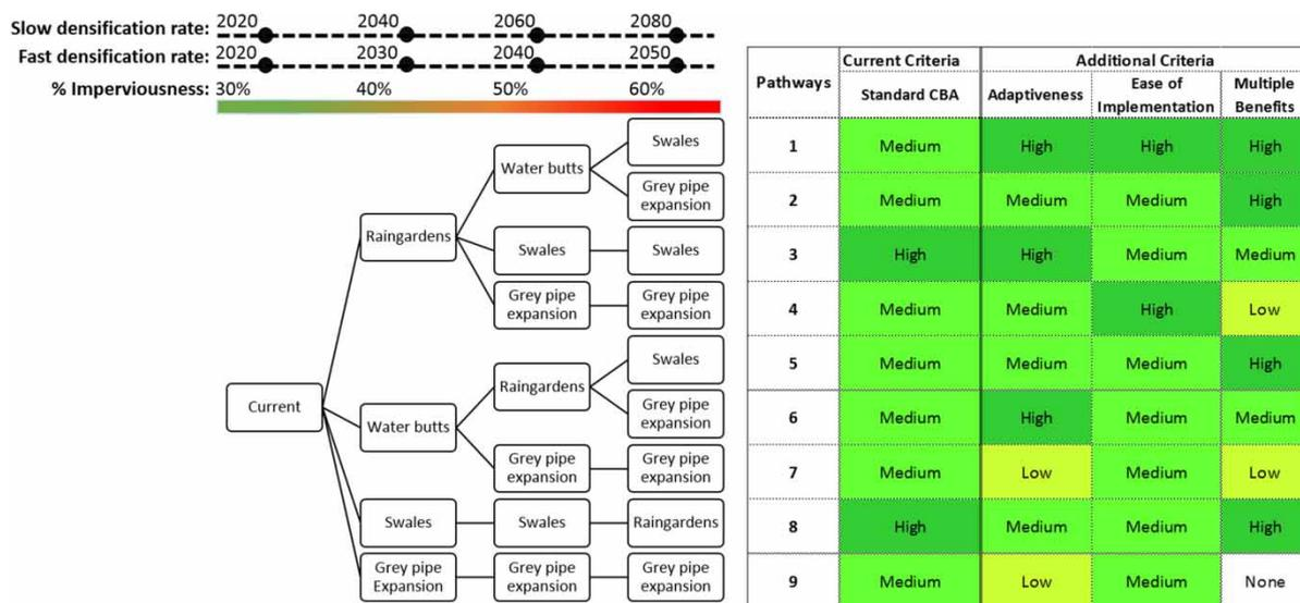
**Figure 3** | Adaptation pathways tree and multi-criteria pathway assessment as a response to different rates of urbanisation. Tipping points are identified when the (future) system reaches a capacity threshold due to urban densification pressure, as expressed by an increasing % imperviousness of the urban catchment. A fast or slower rate of densification suggest that the next step should be taken sooner or later, respectively. CBA, cost benefit analysis.
