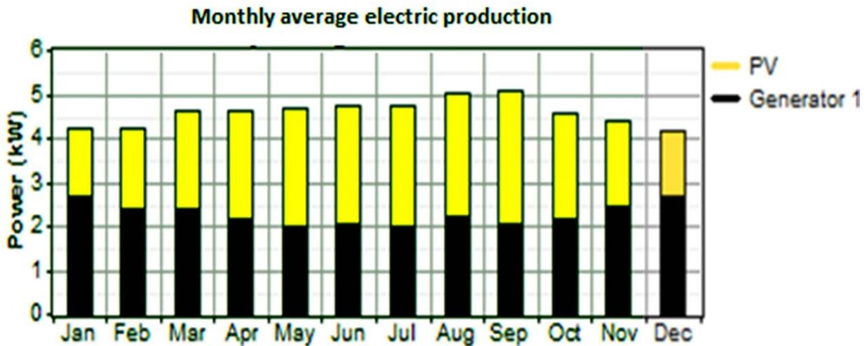
Figure 7. Electric production by PV-Generator system in different months for Zanzan
