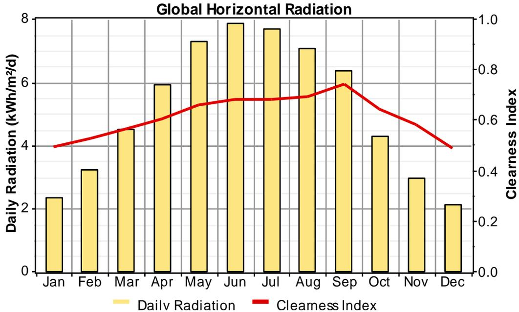
Figure 5. Global horizontal radiation for Zanjan city
