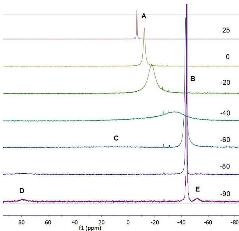
**Figure 2.** Variable-temperature  $^{31}\text{P}\{^1\text{H}\}$  NMR spectra of **1Ge** in  $d_8$ -toluene.
