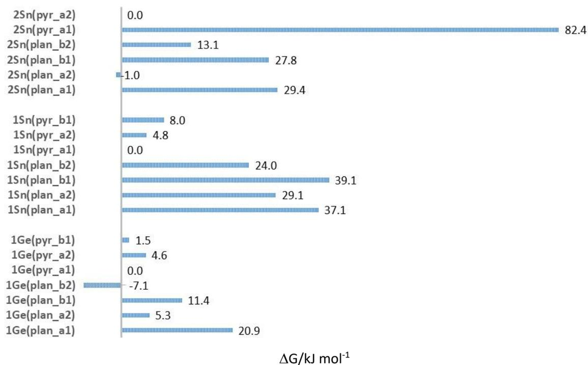
**Figure 9.** Relative free energies of the calculated geometries of **1Ge**, **1Sn**, and **2Sn** (values in kJ mol<sup>-1</sup> are relative to the geometry corresponding to the solid state structure in each case).
