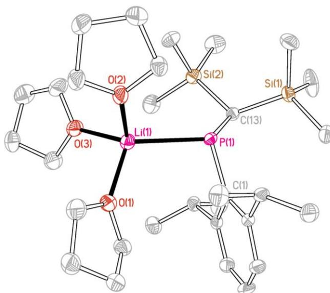
**Figure 4.** Molecular structure of **2Li** with H atoms omitted for clarity. Selected bond lengths (Å) and angles (deg.): P(1)-Li(1) 2.563(4), P(1)-C(1) 1.851(2), P(1)-C(13) 1.909(2), Li(1)-O(1) 2.000(4), Li(1)-O(2) 1.982(4), Li(1)-O(3) 1.990(4), Li(1)-P(1)-C(1) 103.86(11), Li(1)-P(1)-C(13) 127.90(11), C(1)-P(1)-C(13) 105.24(10).
