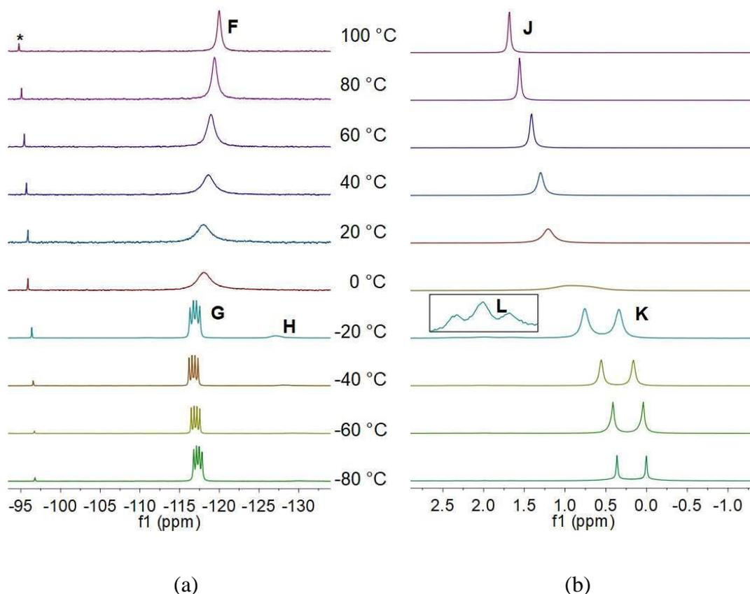
**Figure 5.** Variable-temperature (a)  $^{31}P\{^1H\}$  and (b)  $^7Li$  NMR spectra of **2Li** in  $d_8$ -toluene (\*free phosphine **2H**).
