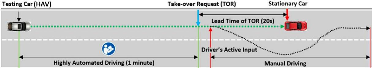
Figure 2 –Illustration of the HAV scenario (Li et al., 2018; Li et al., 2019a).
