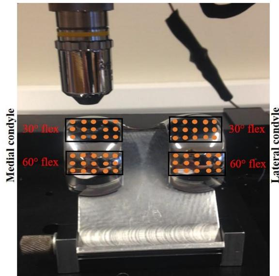
**Figure 4:** Representation of 60 roughness measurements made at two different flexion angles on the femoral component with 30 measurements carried out on each condyle
