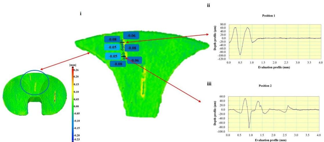
**Figure A.1** (i) Deviation values shown at different positions of an intentional scratch on the non-bearing region of the component; depth profile obtained at (ii) position 1 (iii) position 2 of a scratch
