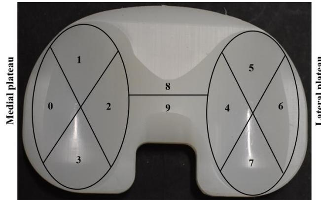
**Figure 3:** The articular surface of the PE insert was divided into 10 different regions for damage mode assessment
