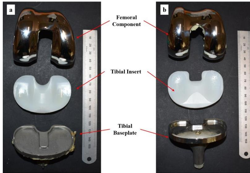
**Figure 1:** (a) Stryker Triathlon (Femoral component – Cobalt-Chromium (CoCr) alloy, Tibial Insert – XLPE, Tibial baseplate – non-polished CoCr); (b) DePuy Sigma (Femoral component – CoCr alloy, Tibial Insert – CPE, tibial baseplate – polished CoCr)
