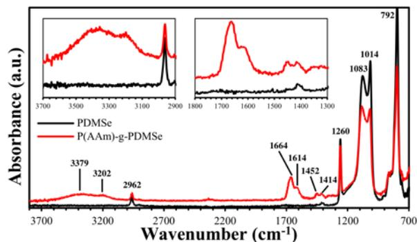
**Figure 1.** ATR-FTIR spectra of as-cured PDMS<sub>e</sub> (black) and P(AAm)-g-PDMS<sub>e</sub> (red). P(AAm) grafting is evidenced by new peaks corresponding to the amide I and II and primary amine absorption bands (insets) of P(AAm) that are not present in as-cured PDMS<sub>e</sub>.
