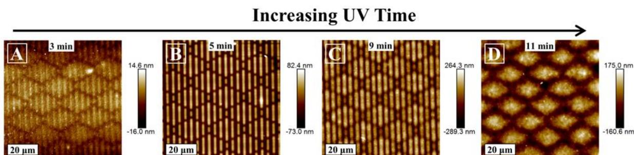
**Figure 5.** 2D AFM scans of SK2x2\_n4 P(AAm)-g-PDMSe with increasing UV polymerization time showing the onset of pattern formation at 3 min after the RAFT inhibition period, followed by high-fidelity patterns from 3-8 min, and proceeding to gradual thickening of the patterns at 9 min with complete loss of independent features at 11 min.
