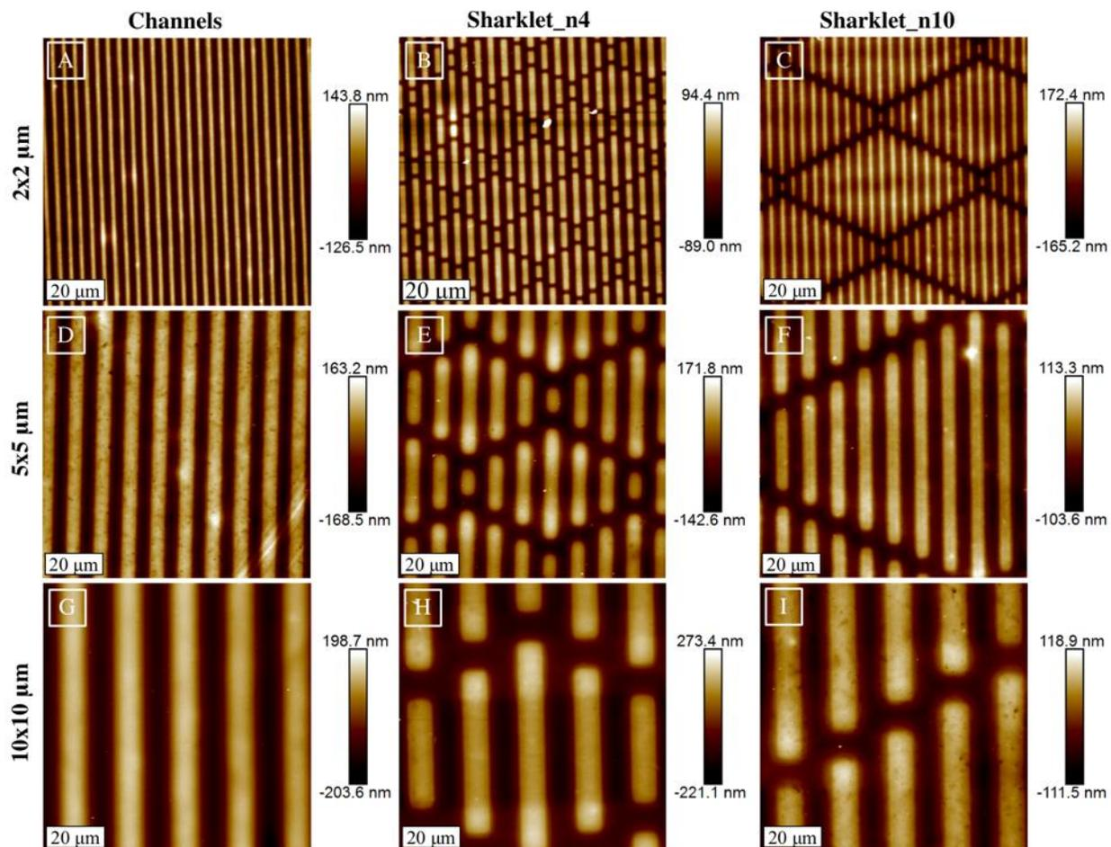
**Figure 2.** Representative 2D AFM height sensor scans of P(AAm)-g-PDMSe surfaces immersed in DIW. (A) CH2x2, (B) SK2x2\_n4, (C) SK2x2\_n10, (D) CH5x5, (E) SK5x5\_n4, (F) SK5x5\_n10, (G) CH10x10, (H) SK10x10\_n4, and (I) SK10x10\_n10. Each row represents a different lateral spacing group (2x2, 5x5, or 10x10  $\mu\text{m}$ ) and each column represents different pattern geometries (Channels, Sharklet\_n4, or Sharklet\_n10). All scans are approximately 93x93  $\mu\text{m}^2$ .
