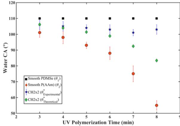
**Figure 4.** Water CA vs. UV polymerization time for experimentally measured surfaces including non-patterned P(AAm) ( $\theta_2$ , red), CH2x2 ( $\theta_{experimental}^*$ , blue), and the theoretically predicated composite CA ( $\theta_{theoretical}^*$ , green) assuming a constant non-grafted PDMSe CA of 110° ( $\theta_1$ , black) according to Eq. 1. Experimental data points represent the arithmetic average ( $\pm$  standard deviation), N=3, n=5
