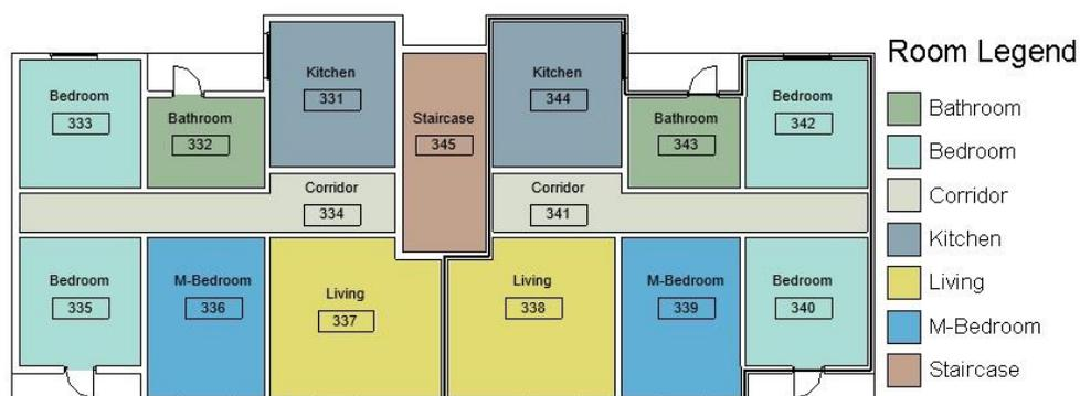
**Figure 4.** Spaces and zones identification in BIM (Revit)
