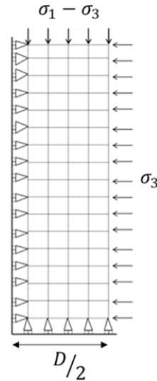
Fig. 4 The finite element mesh and boundary condition based on [1]
