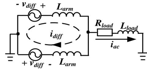
Figure 4: Common and differential mode of MMC leg
