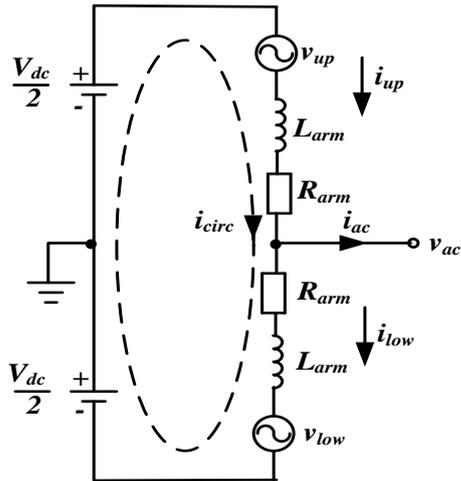
Figure 3: Equivalent circuit of one phase of MMC
