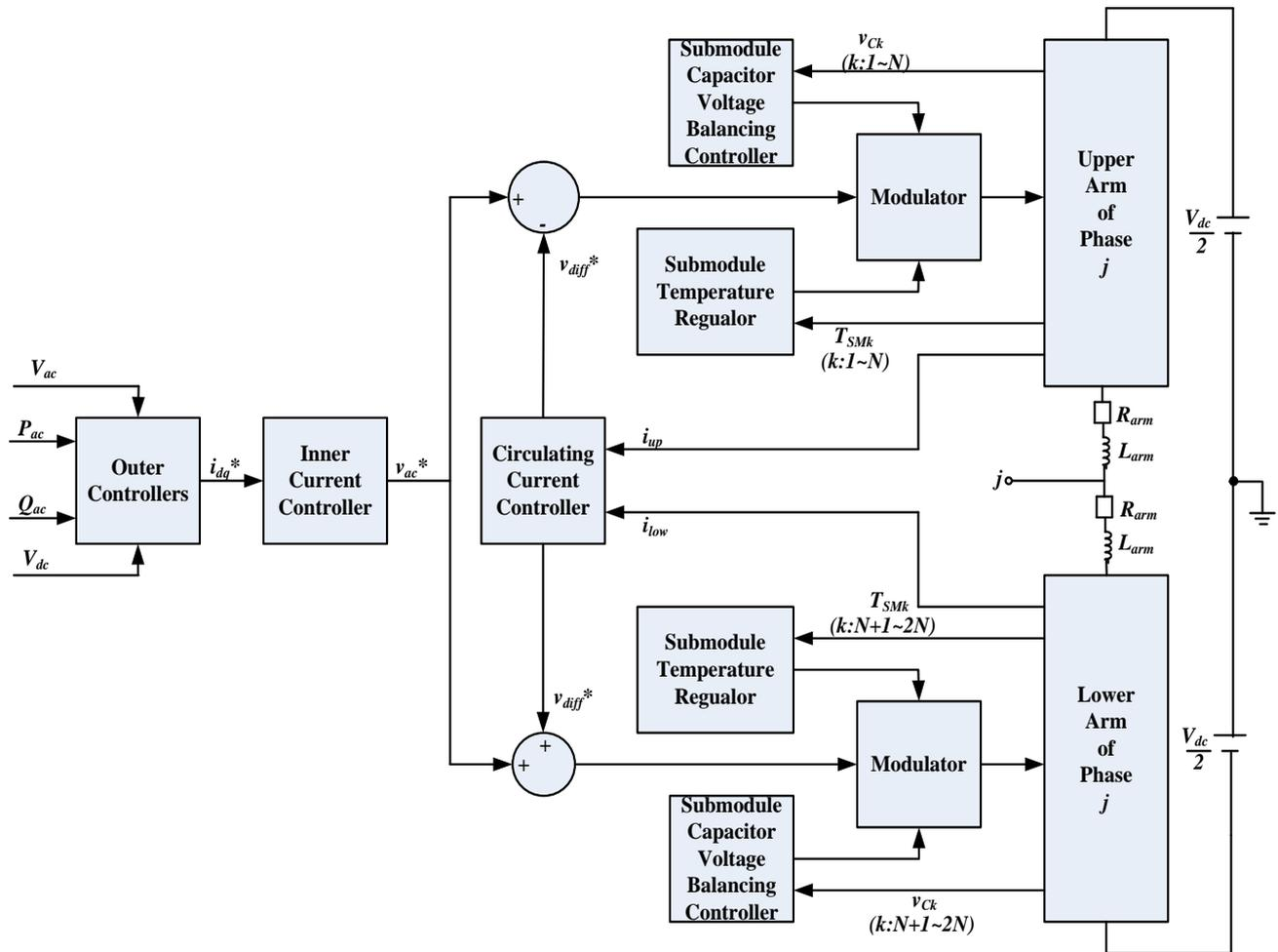
Figure 1: Block diagram of MMC Control loops
