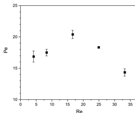
Figure 2. Peclet number (Pe) at different Re in a serpentine microchannel with 2 mm hydraulic diameter.
