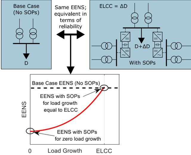
Fig. 1. The main concept of the ELCC methodology for soft open points.
