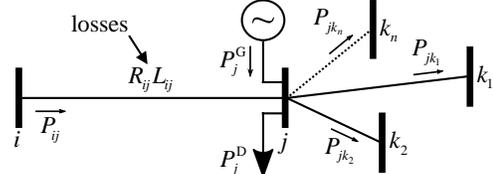
Fig. 3. Graphical representation of the *DistFlow branch equations*. The (active / reactive) power flow at the sending node of branch  $ij$  is equal to the sum of: i) sum of power flows from node  $j$  to nodes  $k_1, k_2, \dots, k_n$ , ii) branch losses, iii) demand at node  $j$ , and iv) minus generation at node  $j$ .
