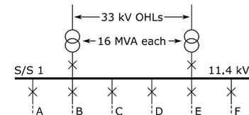
Fig. 5. The upstream network circuits that supply S/S 1 of the TPC DN.
