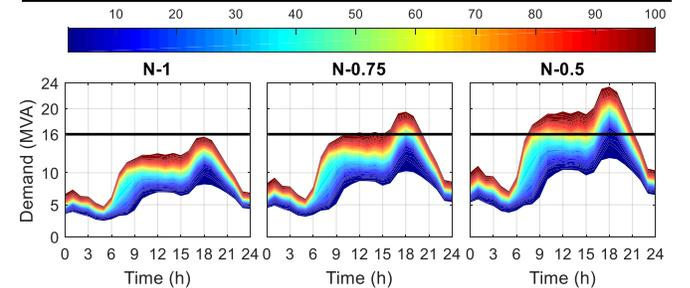
Fig. 6. Substation S/S 1 loading level for each redundancy level (winter). The colour bar indicates the cumulative probability of each loading level. The black line represents the capacity of a single transformer.
