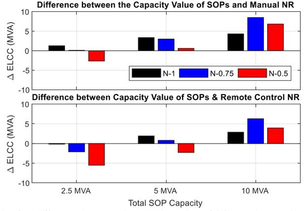
Fig. 8. Difference between the capacity value of SOPs and manual/remote control network reconfiguration.  $\Delta ELCC = ELCC_{SOP} - ELCC_{NR}$ .
