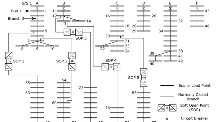
Fig. 4. The modified TPC DN. Substation S/S 1 supplies feeders A–F; substation S/S 2 supplies feeders G–K.
