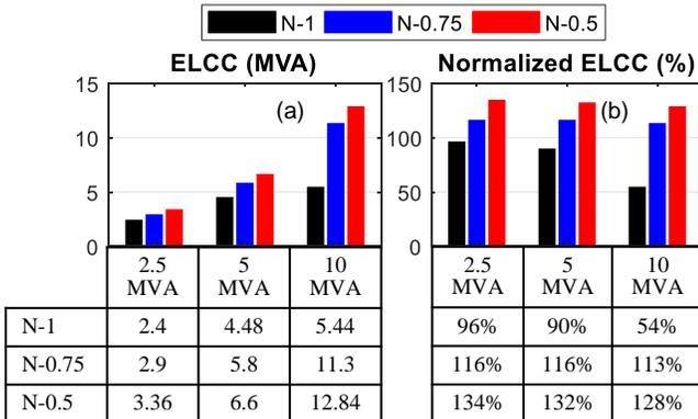
Fig. 7. ELCC in MVA (a), and normalized ELCC (b) (percentage of total SOP capacity) versus total SOP capacity (2.5 MVA, 5 MVA, and 10 MVA) for three redundancy levels (N-1, N-0.75, and N-0.5).
