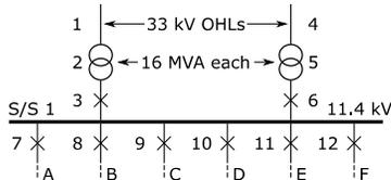
Fig. 9. Substation S/S 1 incoming circuits (with numbered components).
