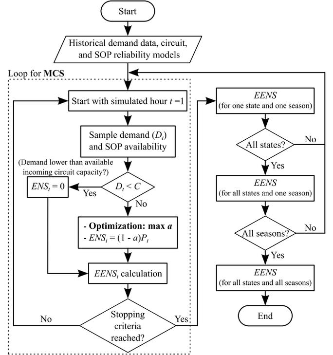
Fig. 2. Overview of the MCS algorithm used to evaluate system reliability.
